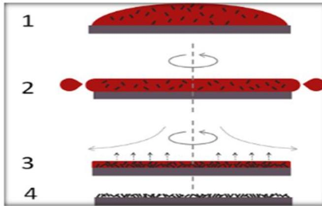
*Figure 2.2.* Spin coating for a little molecule in solution by a static dispense
