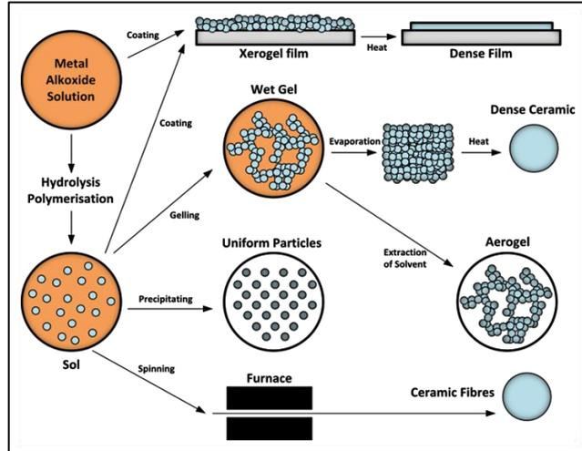
*Figure 2.1. Process of Sol-gel Technology and Products*
