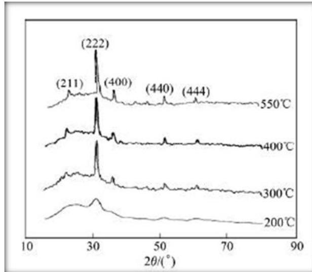
*Figure 2.3.* XRD patterns of ITO films heat-treated at various temperatures
