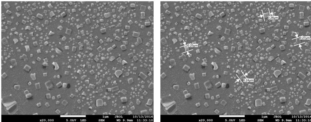
*Figure 4.3.* The morphologies of ITO thin film annealed at 300 °C with 20 000x Magnification
