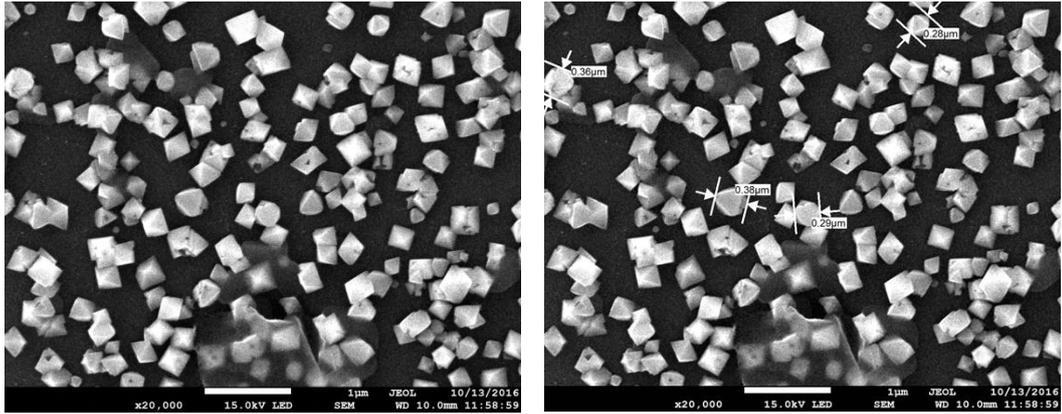
Figure 4.4. The morphology of ITO thin film with annealed at 400 °C with 20 000x Magnification
