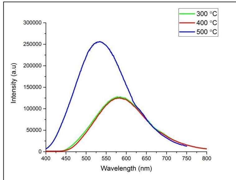
*Figure 4.8.* PL spectra of ITO thin films annealed at 300 °C, 400 °C and 500 °C respectively
