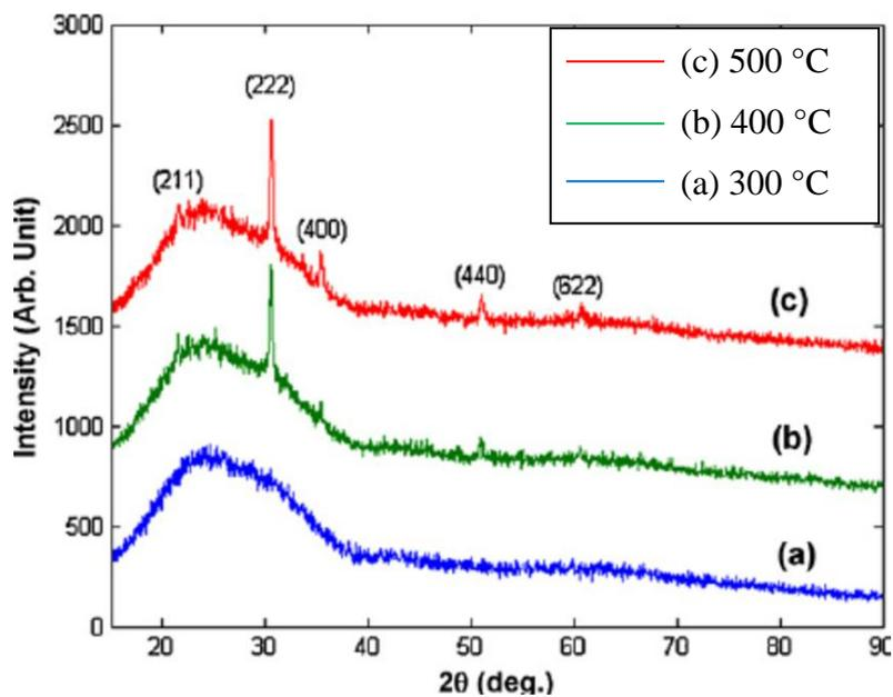
Figure 4.2. XRD spectra of ITO thin films annealed at 300 °C, 400 °C and 500 °C respectively
