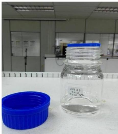
Figure 4.1. Precursor of ITO solution after leaving for aging
