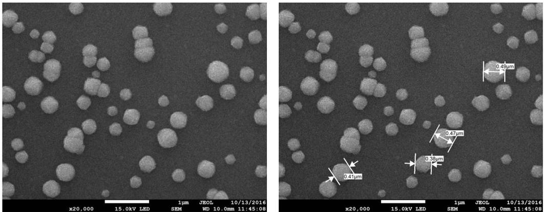
Figure 4.5. The morphology of ITO thin film annealed 500 °C with 20 000x Magnification
