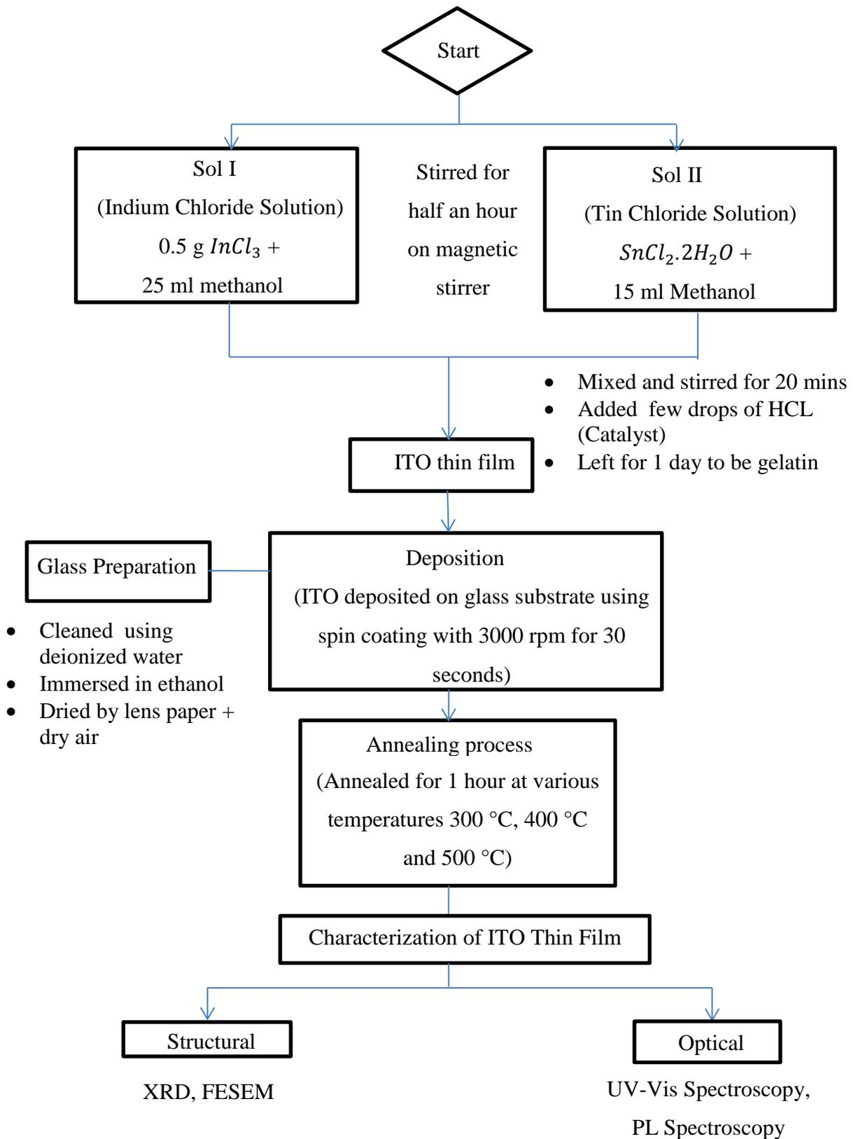
Figure 3.1. The flowchart of the guidelines for the laboratory experimental work
