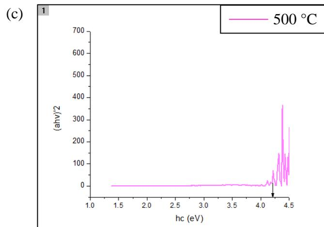
Figure 4.7. The plot of  $(\alpha h\nu)^2$  against  $(h\nu)$  of ITO thin films annealed at 300 °C, 400 °C and 500 °C respectively
