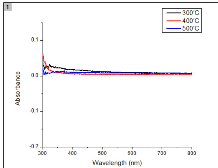
*Figure 4.6.* Absorbance versus wavelength spectra of ITO thin films annealed at various temperatures annealed at 300 °C, 400 °C, and 500 °C respectively
