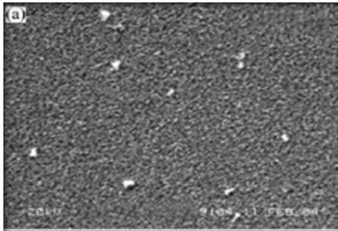
*Figure 2.4.* SEM surface photos of ITO films heat-treated at 600 °C
