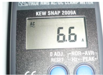
Figure 5.6: Current Draw after APFC operated (1.32KW).
