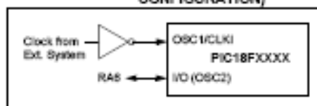
FIGURE 2-5: EXTERNAL CLOCK INPUT OPERATION (ECIO AND ECPIO CONFIGURATION)
