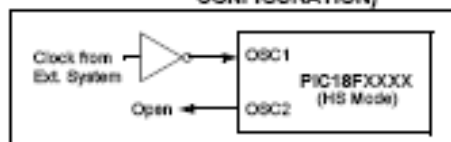
FIGURE 2-3: EXTERNAL CLOCK INPUT OPERATION (HS OSC CONFIGURATION)
