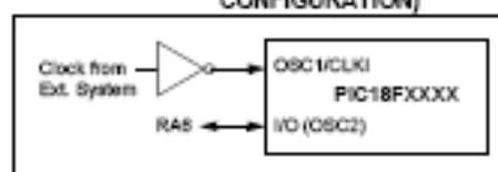
FIGURE 2-5: EXTERNAL CLOCK INPUT OPERATION (ECIO AND ECP10 CONFIGURATION)
