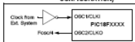
FIGURE 2-4: EXTERNAL CLOCK INPUT OPERATION (EC AND ECP10 CONFIGURATION)
