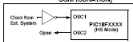
FIGURE 2-3: EXTERNAL CLOCK INPUT OPERATION (HS OSC CONFIGURATION)
