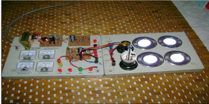
FIGURE 4.3: LED Power Saving is in ON state state and the meter are showing the voltage and current reading
