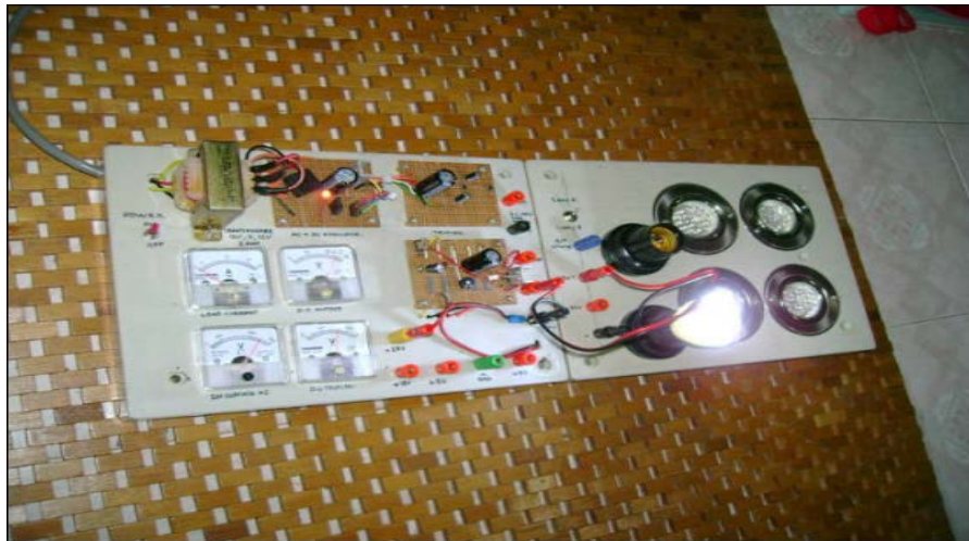
FIGURE 4.4: LED Bulb is in ON state and the meter are showing the voltage and current reading
