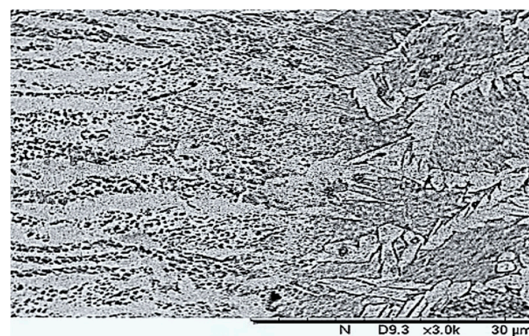
Figure 15. SEM of weld microstructures at a point near 2205 side.
