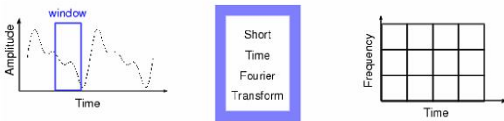
Figure 4: Short-Time Fourier Transform of a Time Series Signal (Figure obtained from MATLAB help file)
