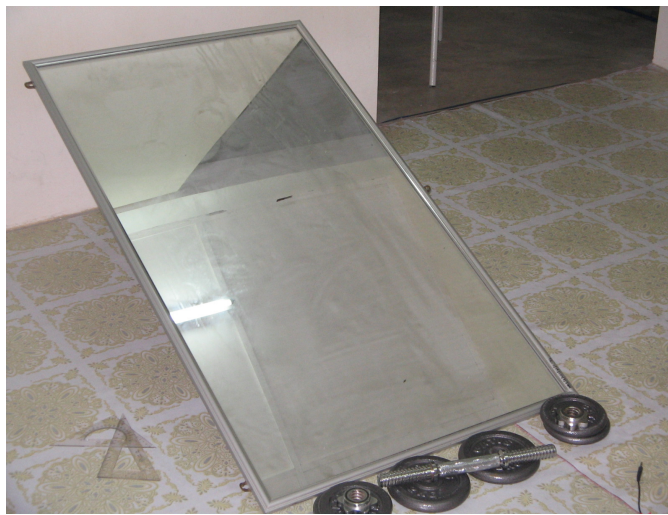
Figure 4.11: Test window with size 660 mm x 1150 mm
