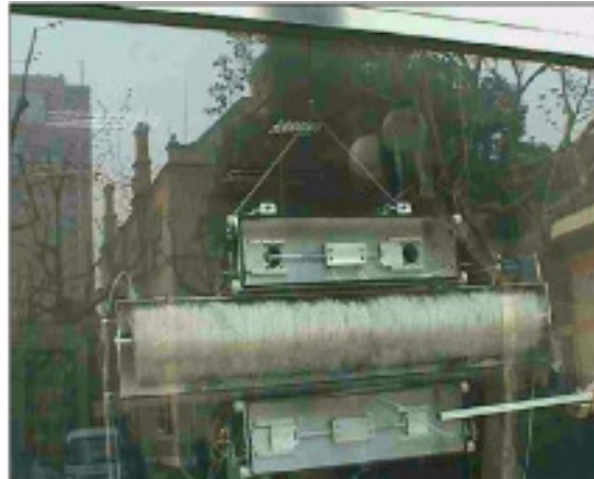
Figure 2.13: Wall-climbing robots with sliding suction cups
