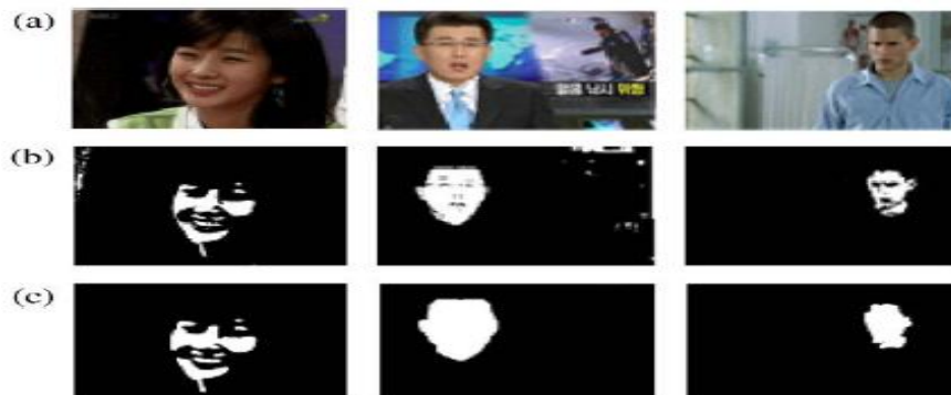
Figure 2.13: Morphological image processing. (a) Original images. (b) Skin tone detected images. (c) Results of the closing process.
