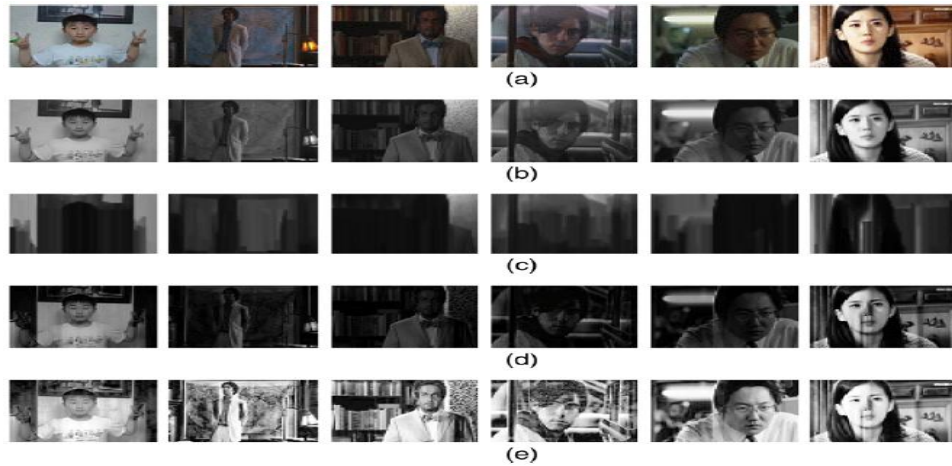
Figure 2.10: Examples of the illumination-compensation. (a) Original images. (b) Y component images. (c and d) Bilinear interpolated images by the minimal value in 20 x 20 window. (e) Illumination-compensated images.
