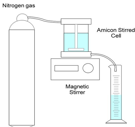
Figure 1: Experimental set up (Amicon stirred cell, model 8200)
