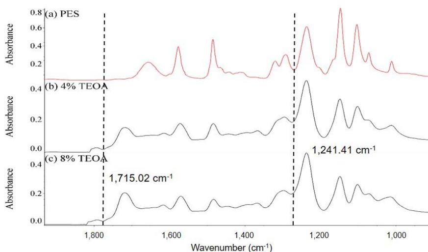
Figure 2: ATR-FTIR spectra of TFC membrane
