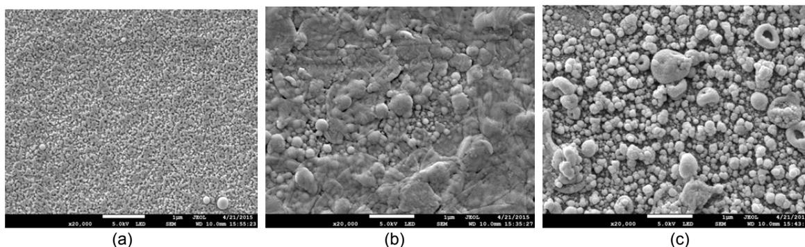
Figure 3: FESEM images of surface of (a) UF PES (20,000 $\times$  magnification), (b) 4 % TEOA (20,000 $\times$  magnification) and (c) 8 % TEOA (20,000 $\times$  magnification)
