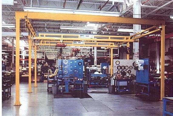
**Figure 1.5:** Overhead crane
