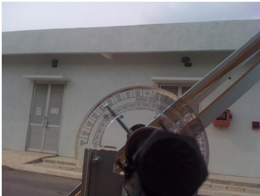
Figure 3.6: Protractor used to read the elevation angle of the dummy solar tracker.
