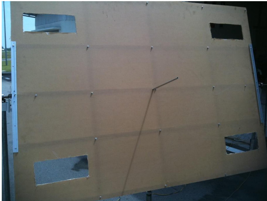
Figure 4.5: Example of shadow from shadow indicator without active tracking.
