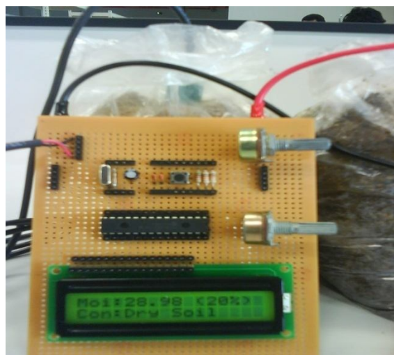
Figure 4.7: Value on LCD screen when tested with dry soil
