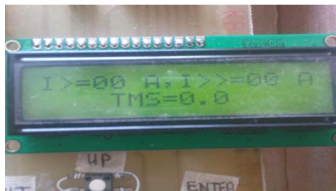
Figure 4.9: LCD display the setting value
