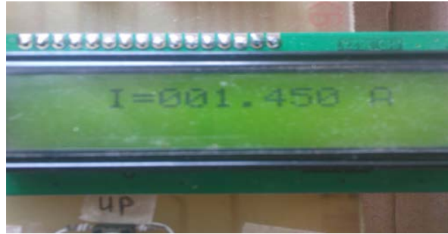
Figure 4.11: LCD display the load current
