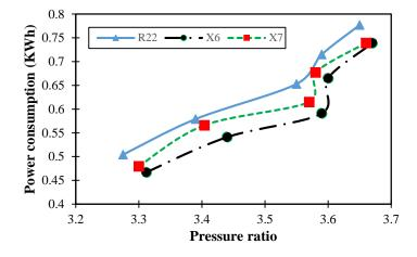
Figure 7. Relationship between power consumption and pressure ratio.
