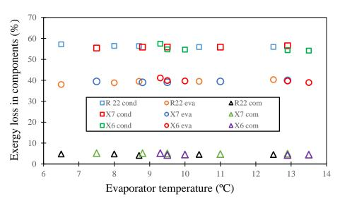
Figure 10. Percentage exergy loss in various components with evaporator temperature.
