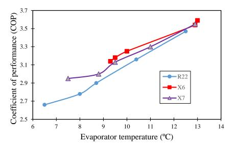
Figure 5. Change in COP with evaporator temperature.
