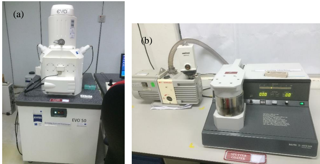
Figure 3. 4. (a) Scanning electron microscope (b) Sputter coater
