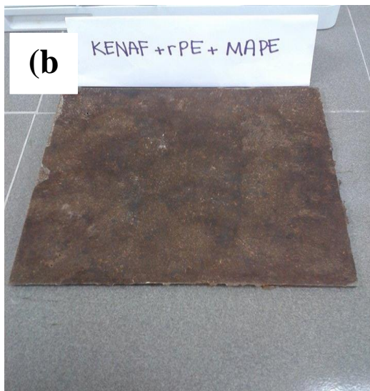
Figure 3.1. The (a) single-screw extruder, (b) kenaf/rPE/MAPE (c) kenaf/rPE/MAPE/nanoclay.
