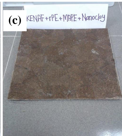
Figure 3.1. The (a) single-screw extruder, (b) kenaf/rPE/MAPE (c) kenaf/rPE/MAPE/nanoclay.
