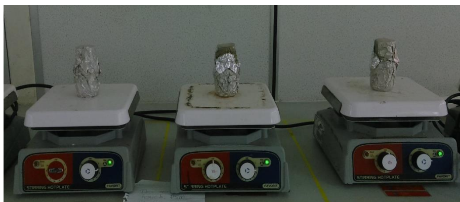
Photograph of CMC/AgNPs heated in dark environment
