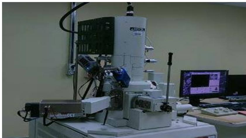
Figure 3.2. Field Emission Scanning Electron Microscope. Source: Purchased from (JEOL JSM-7800F)
