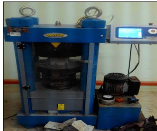
Figure 3. Concrete mixes was filled in cube mould. Figure 4. Compressive strength test in progress.
