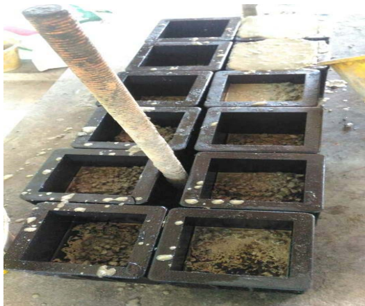
Figure 3. Concrete mixes was filled in cube mould. Figure 4. Compressive strength test in progress.
