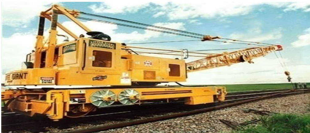
Figure 1.4: Rail Road Crane
