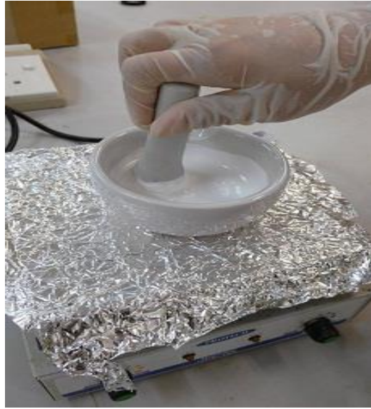
Figure 3.3. Grinding process for mixture of ZnO with ethanol.
