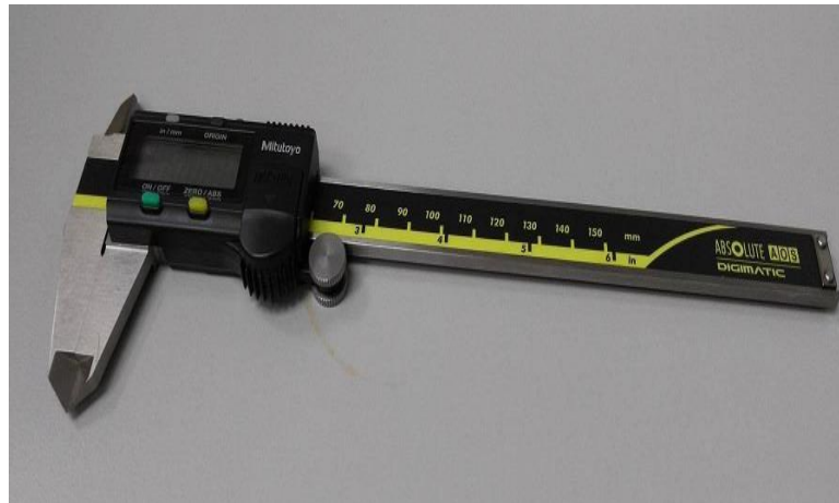
Figure 3.6. Vernier caliper for measuring dimension of ZnO compact bar.
