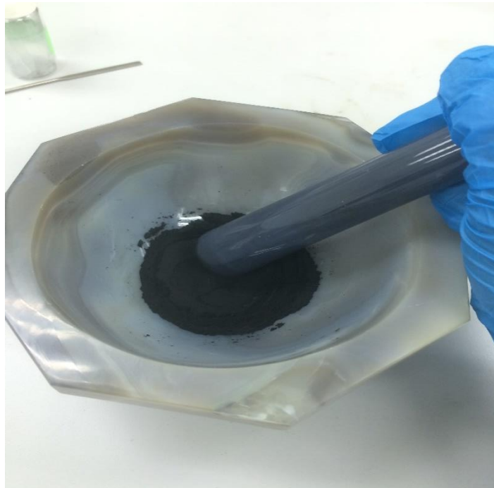
Figure 3.2: Hand grinding using mortar and pestle
