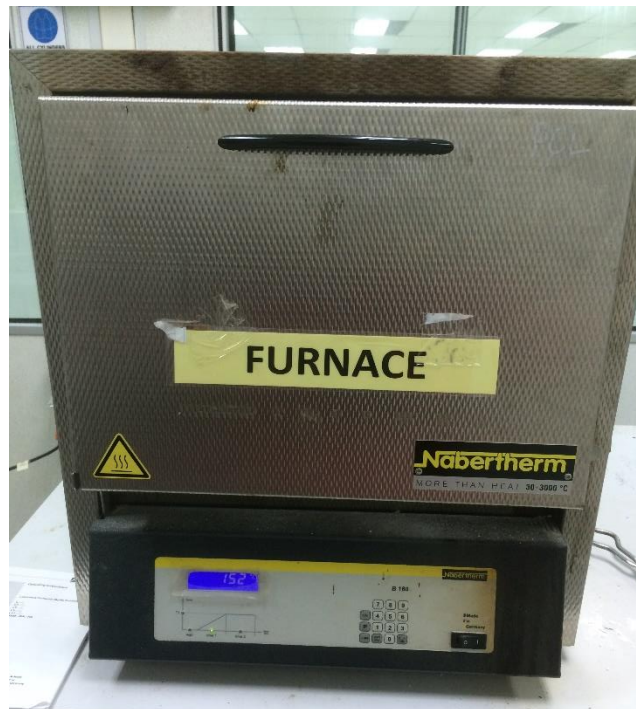
Figure 6: the box furnace used for sintering
