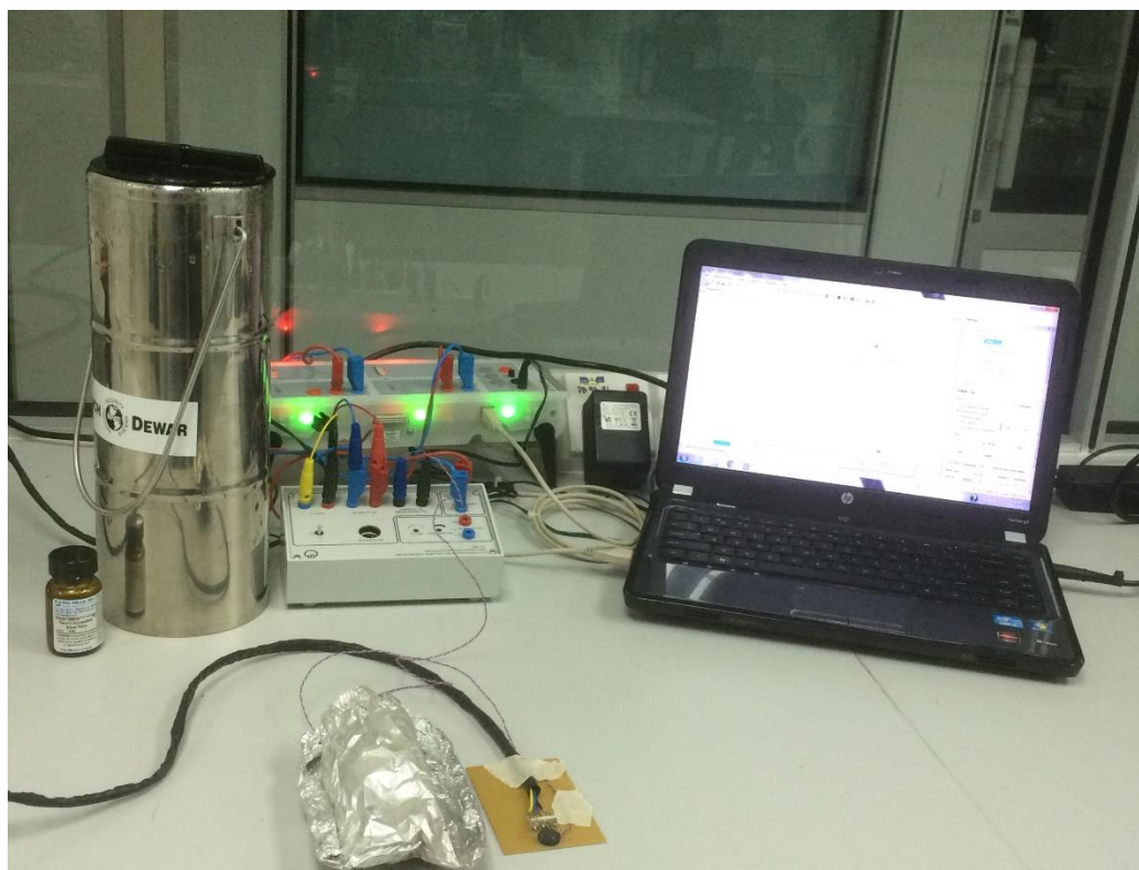
Figure 3.9: The equipment for Four point probe testing.
