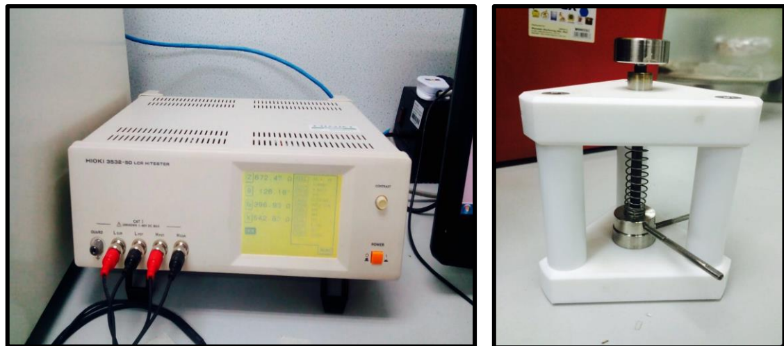
Figure 3.6. The HIOKI 3532-50 LCR Hi-Tester and sample holder
