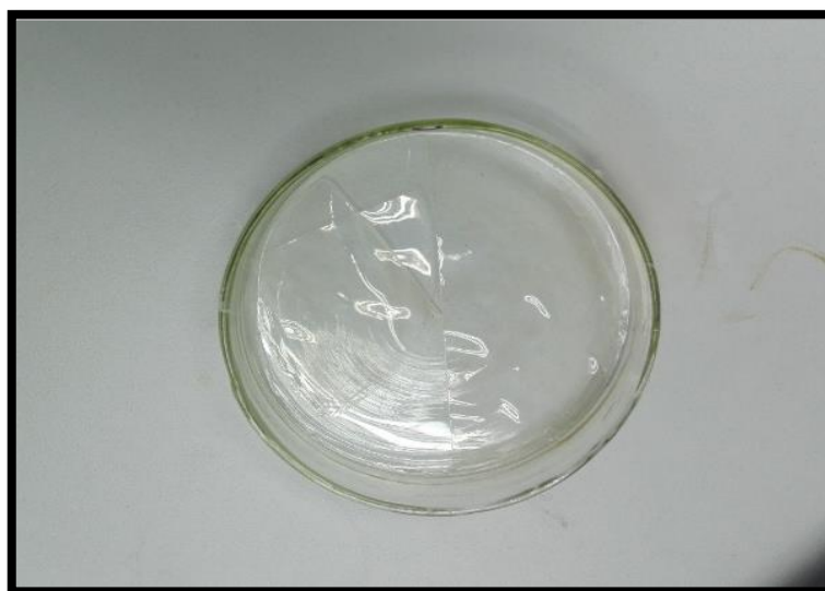
Figure 4.1: Transparent CMC/KC hybrid electrolyte.
