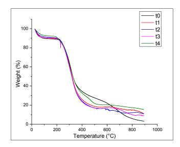
Fig. 3: TGA of untreated and treated chicken feathers.
