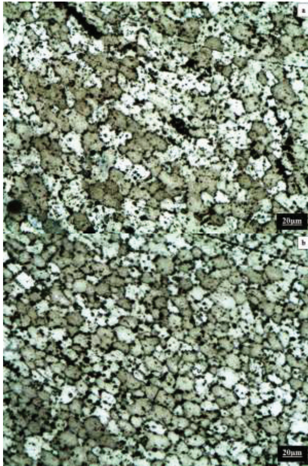
Fig. 1. Microstructure of Stir zone at (a) 70 mm/min (b) 80 mm/min
