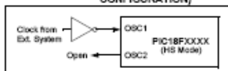
FIGURE 2-3: EXTERNAL CLOCK INPUT OPERATION (HS OSC CONFIGURATION)
