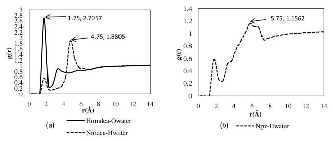
**Figure 5:** Intermolecular interaction of (a) MDEA and water (b) PZ and water for tertiary system of blended MDEA/PZ.
