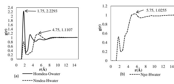
Figure 2: Intermolecular interactions of amine and water in binary system using (a) MDEA and (b) PZ solution.
