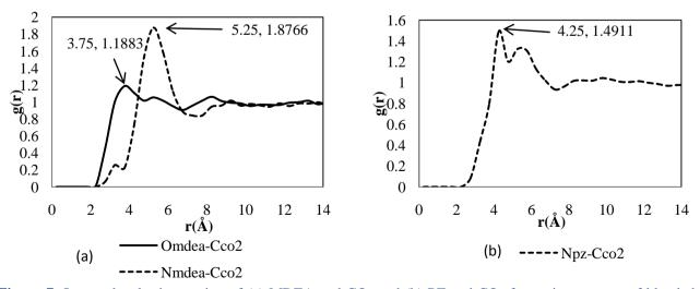
**Figure 7:** Intermolecular interaction of (a) MDEA and CO<sub>2</sub> and (b) PZ and CO<sub>2</sub> for tertiary system of blended MDEA/PZ.
