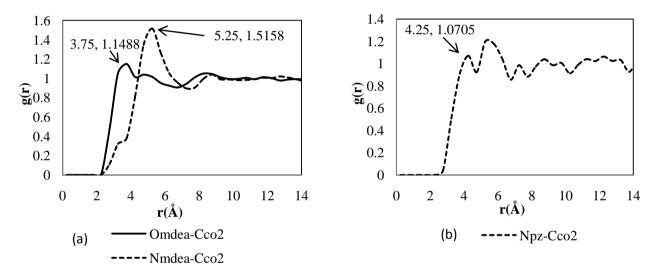
Figure 6: Intermolecular interaction of amine and CO<sub>2</sub> in tertiary system using (a) MDEA and (b) PZ solution.
