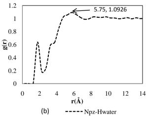
Figure 4: Intermolecular interactions of amine and water in tertiary system using (a) MDEA and (b) PZ solution.
