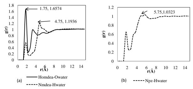
**Figure 3:** Intermolecular interaction of (a) MDEA and water and (b) PZ and water for binary system of blended MDEA/PZ.
