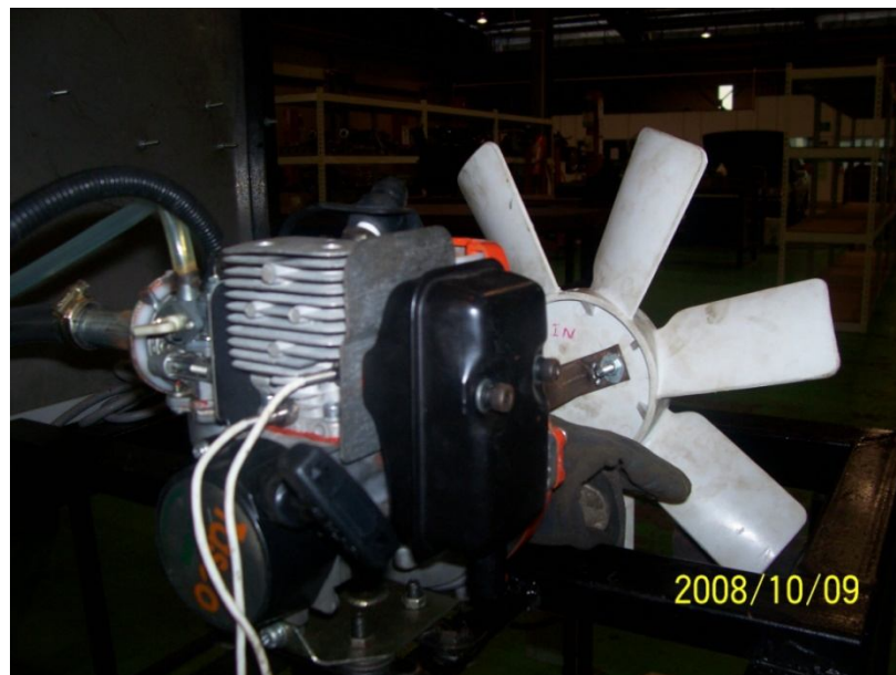
Figure 4.14: The Pressure Sensor Located At Intake and Scavenge Port
