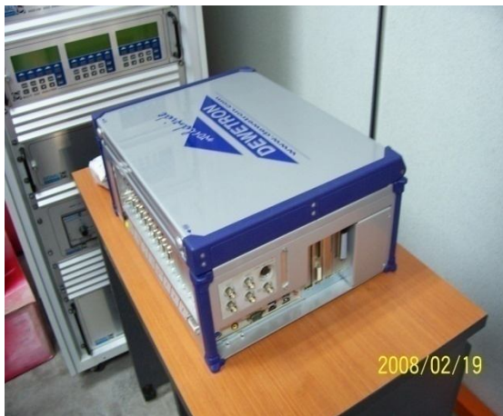
Figure 3.8: Data Acquisition System (DAQ)
