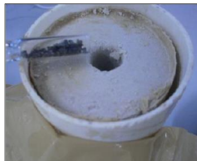
Fig 1 Installation of bottom ash in soft kaolin clay specimen
