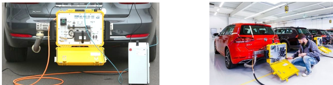
Figure 18. (PEMS) installation on vehicles.
