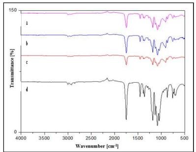
Figure 1: FTIR analysis of photocatalyst (a) AgO/Chitosan<sub>NaOH</sub>, (b) Chitosan only, (c) AgO/Chitosan<sub>HCI</sub>, (d) AgO/Chitosan<sub>H2O</sub>
