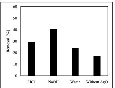
Figure 2: The photcalatys performances of MB using Chitosan<sub>HCl</sub>, Chitosan<sub>NaOH</sub>. Chitosan<sub>H2O</sub> and without AgO. [pH 5; photocatalyst dosage 35 mg L-1; initial concentration 10 mg L-1; stirring speed 1000 rpm].
