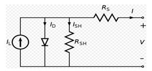
Figure 2.1: The circuit equivalent for a single solar cell
