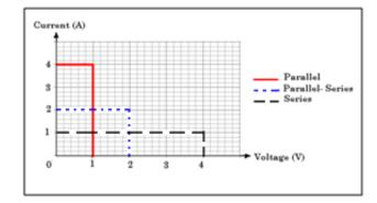
Figure 2.6: Relationship between current and voltage of electrical array reconfiguration
