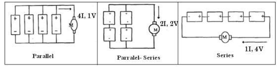
Figure 2.5: Three types of electrical array
