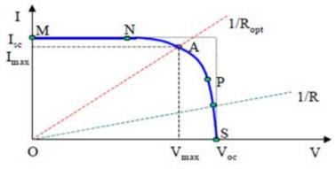
Figure 2.2: A typical current- voltage I-V curve for a PV cell
