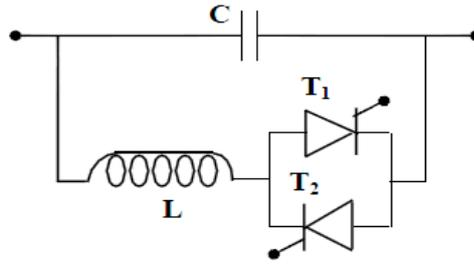
**Fig 2.2:** Basic TCSC circuit
