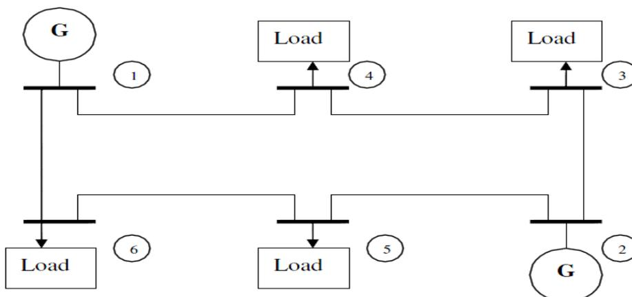
**Fig 3.1:** 6-bus test system diagram
