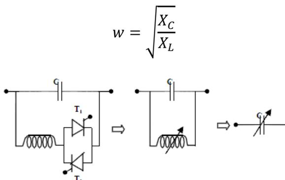
**Fig 2.4:** Equivalent circuit of TCSC
