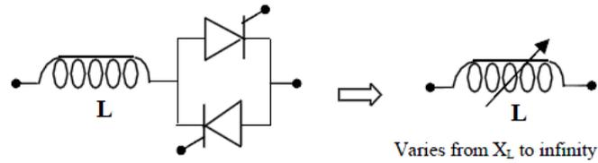
**Fig 2.3:** Simplify of TCSC Circuit
