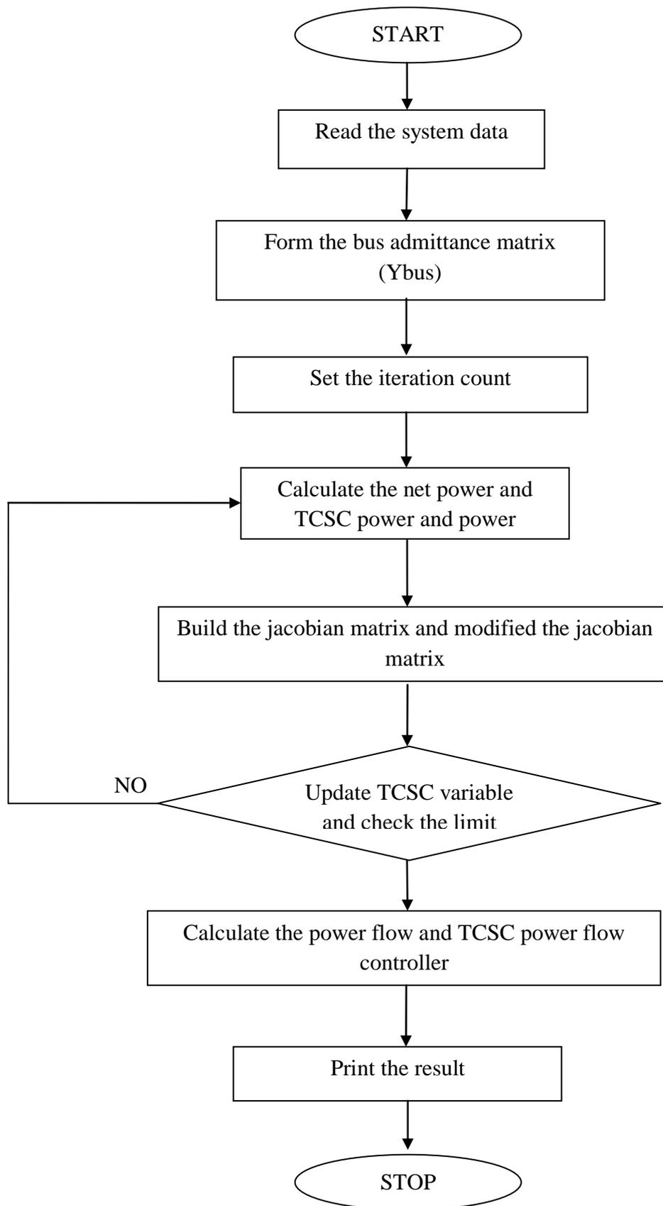
**Fig 3.2:** TCSC Newton-Raphson Flowchart
