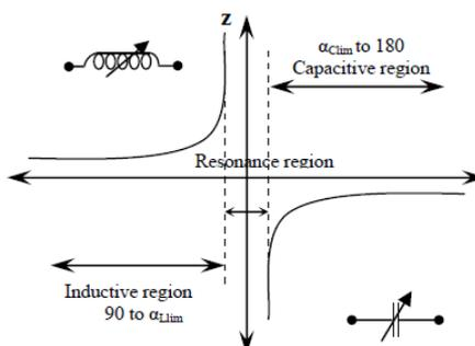
**Fig 2.5:** Impedance Vs firing angle characteristic curve
