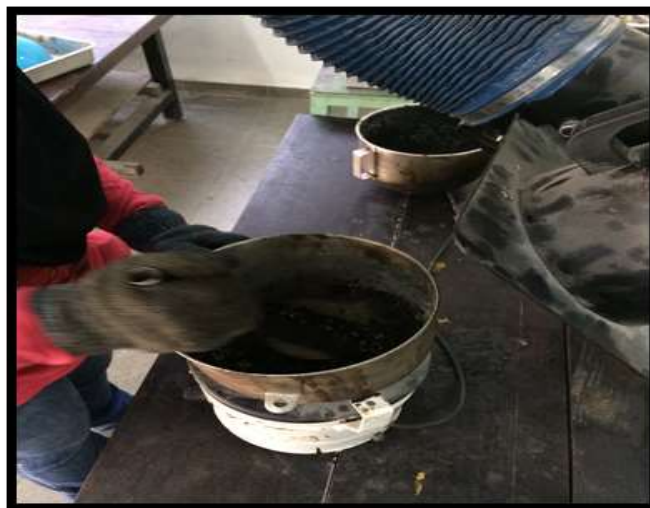
Figure 3.10 Mixed the Asphalt and Aggregate
