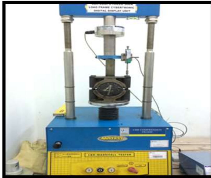
Figure 3.12 Marshall Stability Test Machine
