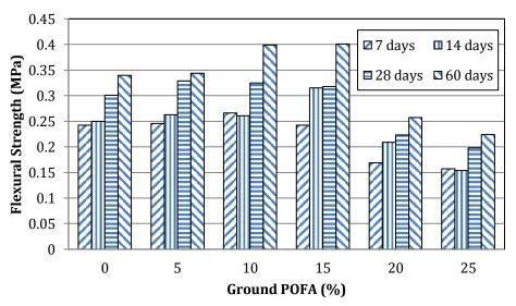
Fig. 4. Flexural strength result of brick with ground POFA content up to 60 days.
