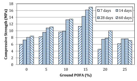
Fig. 3. Compressive strength results of brick with ground POFA content up to 60 days.
