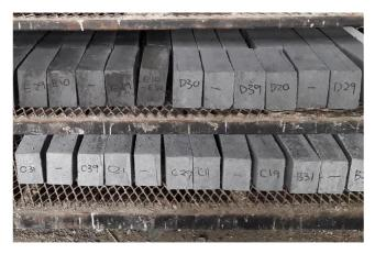
Fig. 2. Sand cement bricks subjected to air curing.
