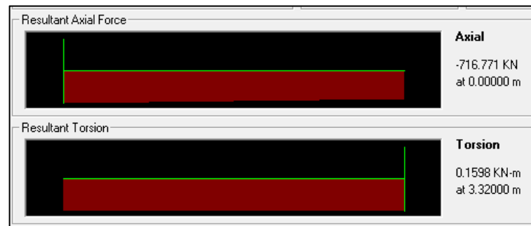
Figure 4.26 Result of axial force and torsion for column 104
