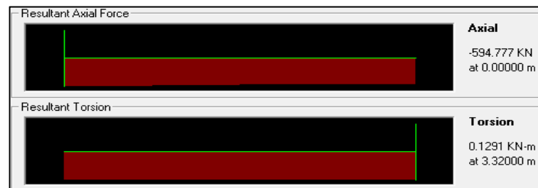
Figure 4.14 Result of axial force and torsion for column 104
