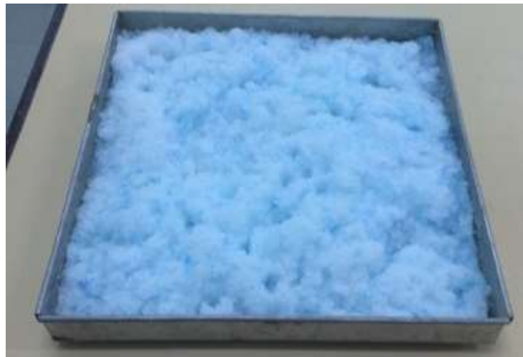
Figure 3.1(a) Superabsorbent polymer before oven drying
