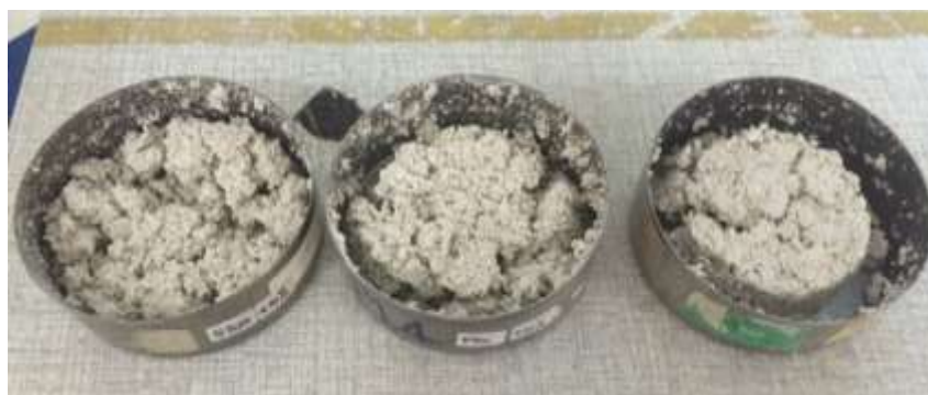
Figure 3.2 Shrinkage limit test for S300, FMC and Speswhite with addition of 10% SAP
