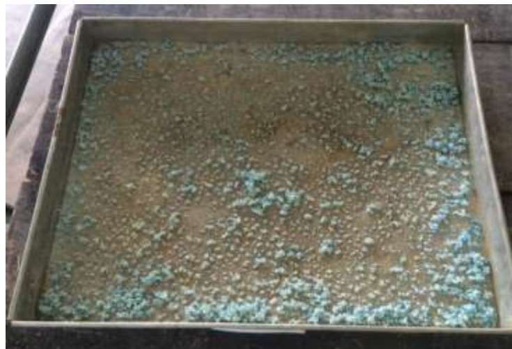
Figure 3.1(b) Superabsorbent polymer after oven drying at 60° c
