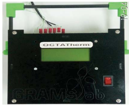
Figure 2. Latest version of temperature data logger system
