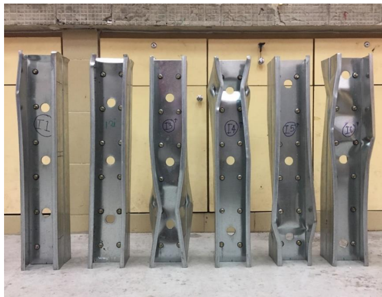
Figure 4.9 The condition of samples after the compression test (Front view)
