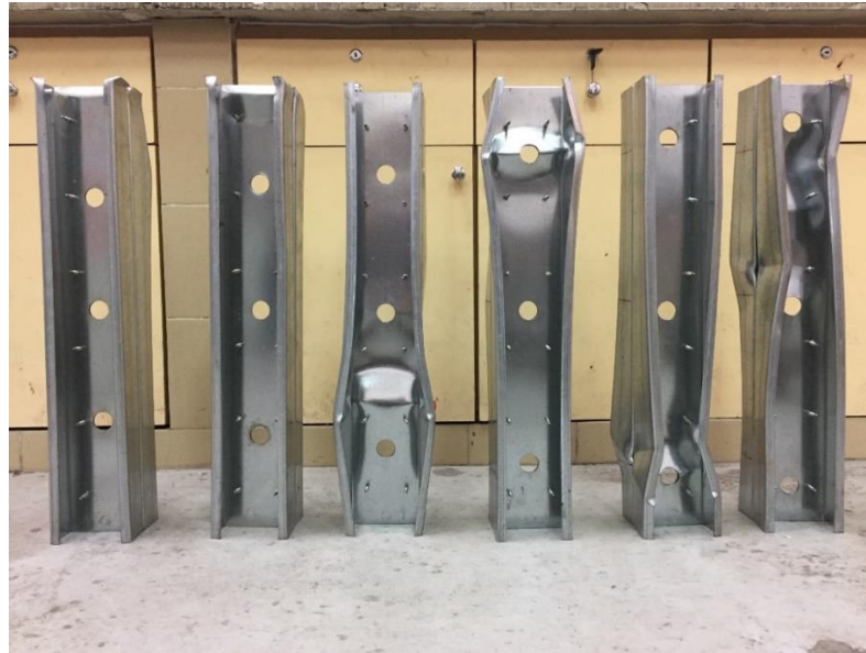
Figure 4.10 The condition of samples after the compression test (Rear view)
