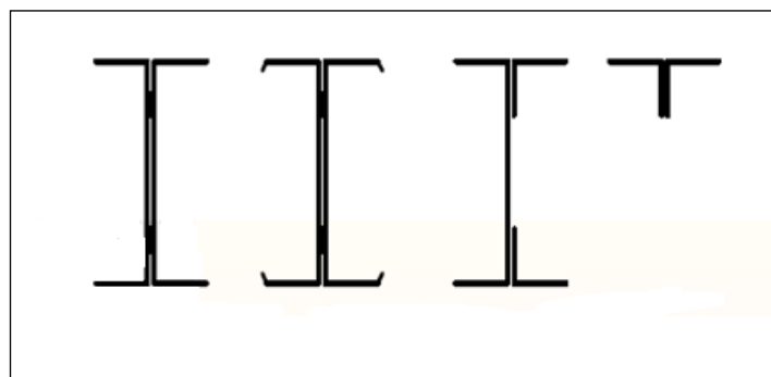
Figure 2.8 Open built-up section
