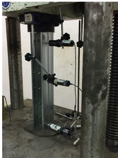
Figure 3.6 The placing of transducer from the side view
