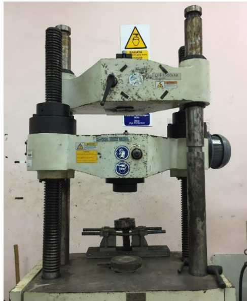
Figure 3.4 Universal testing Machine that are available in FKASA Heavyweight Laboratory
