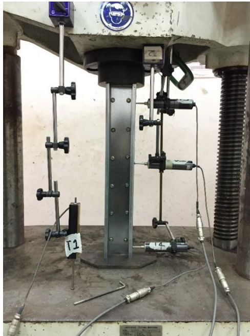
Figure 3.5 The placing of transducer from the front view
