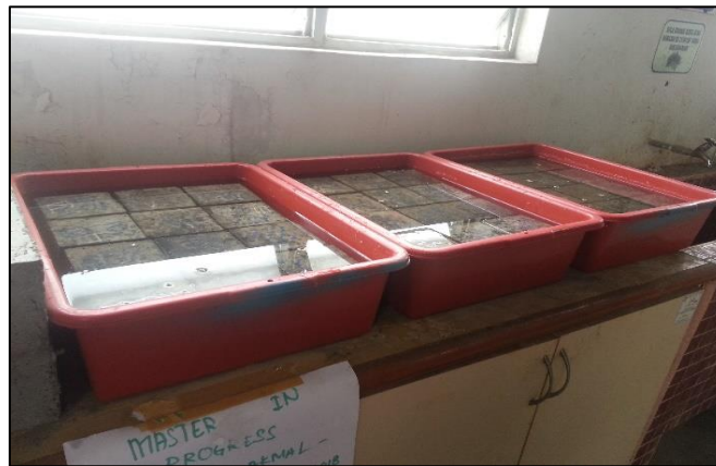
Figure 1. Specimens immersed in sulphate solution.
