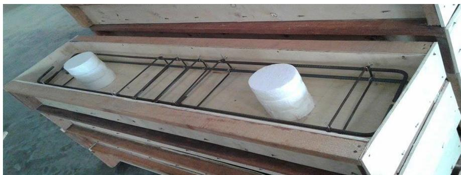
**Figure 3.17:** RC beams with circular openings
