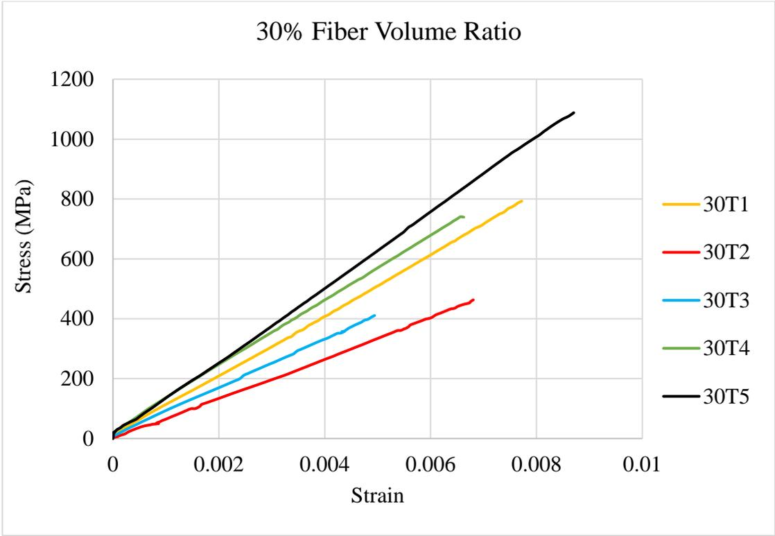
**Figure 4.14:** Stress versus Strain curve in tensile test with 30% fiber volume ratio.
