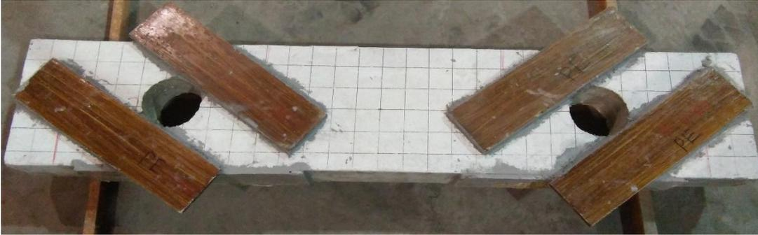
**Figure 3.24:** Surface strengthening with BFRCP for RC circular openings beam.
