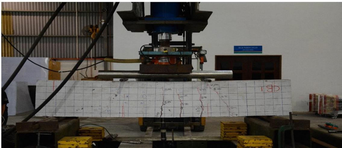
**Figure 3.32:** Setup of four-point loading test
