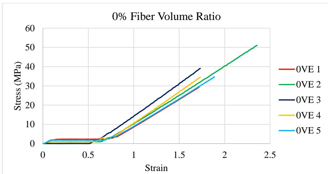
**Figure 4.5:** Stress versus strain curve in flexural test with 0% fiber volume ratio.
