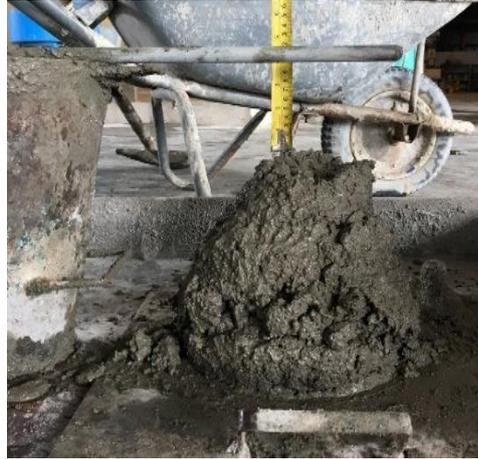
**Figure 4.1:** Slump test
