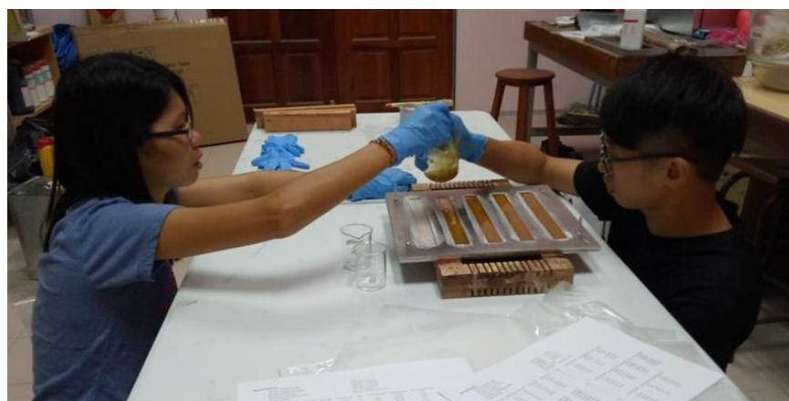
**Figure 3.10:** Fabricating composite plate with hand lay-up method
