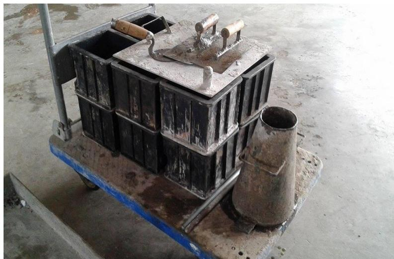
**Figure 3.18:** Tools for slump test and cube test
