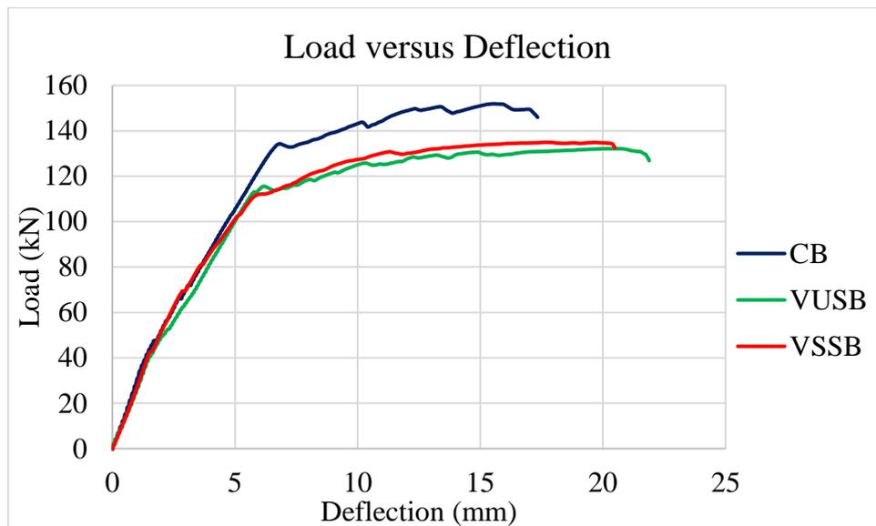
**Figure 4.18:** Load deflection curve of the different beam specimens
