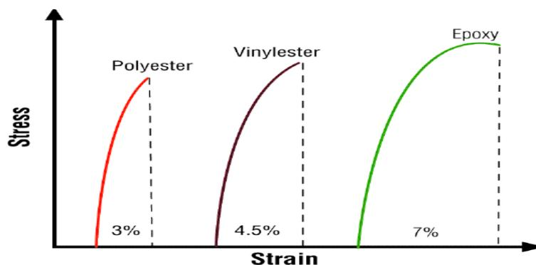
**Figure 2.5:** Comparison of stress versus strain
