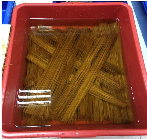
**Figure 3.3:** Soaking of bamboo fiber in warm water
