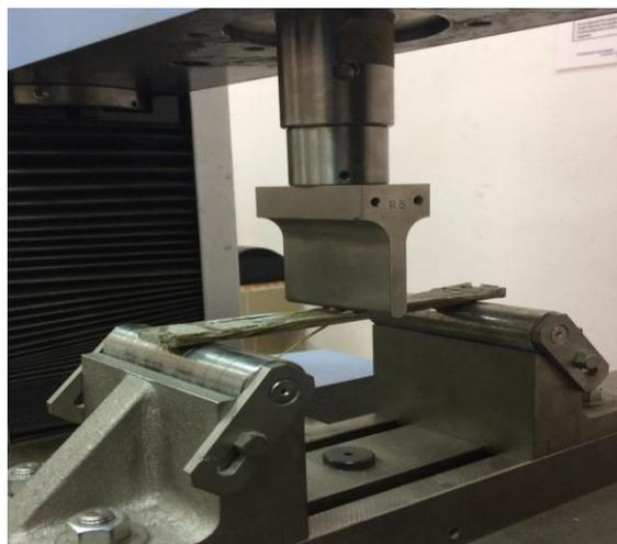
**Figure 3.28:** Flexural test for composite plate
