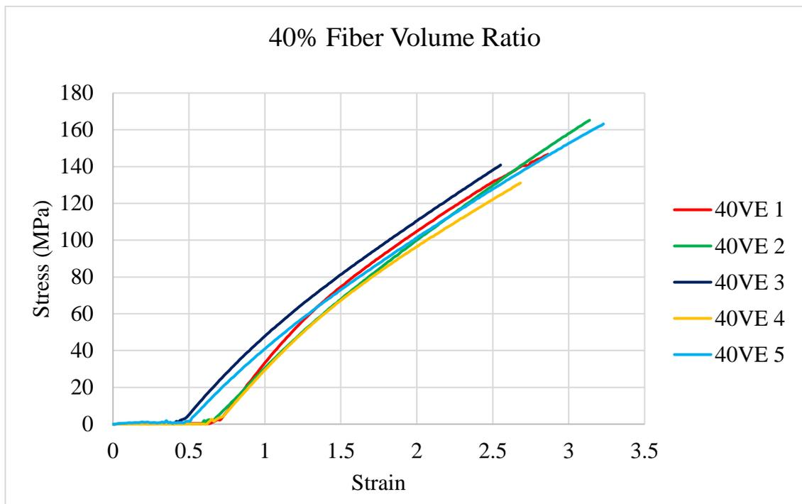
**Figure 4.9:** Stress versus Strain curve in flexural test with 40% fiber volume ratio.
