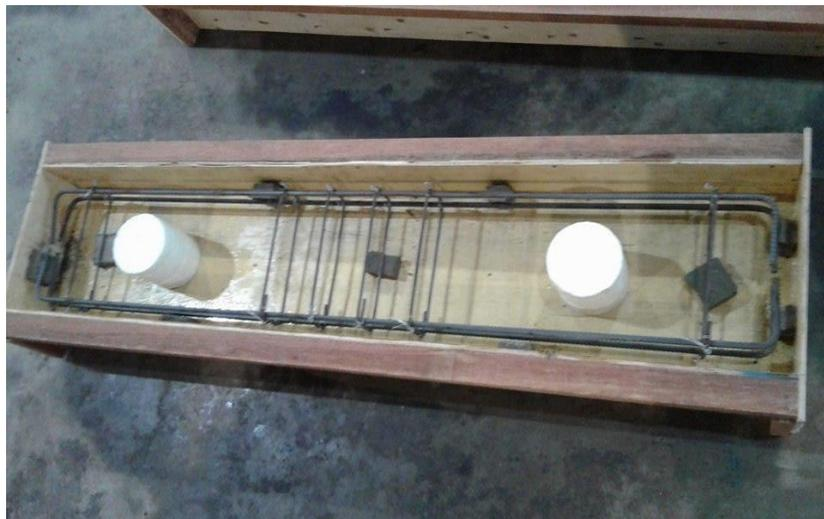
**Figure 3.12:** Formwork for reinforced concrete beams with circular openings
