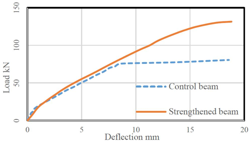
**Figure 2.11:** Load-deflection curve
