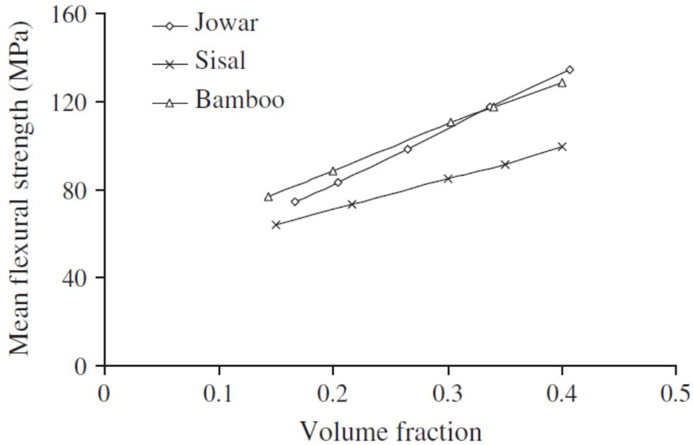
**Figure 2.8:** Effect of volume fraction of fibre for Jowar fibre reinforced composites in comparison to sisal and bamboo fibre composites in flexural test.
