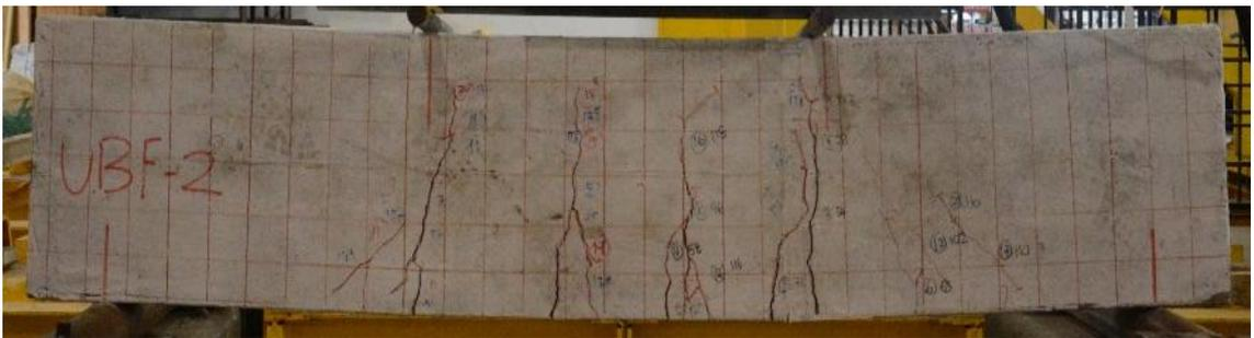
**Figure 4.20:** Crack pattern after failure for un-strengthened solid beam (VUSB)
