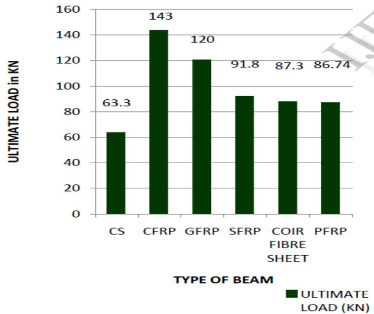
**Figure 2.13:** Comparison of different fiber sheet and control specimen in terms of ultimate load
