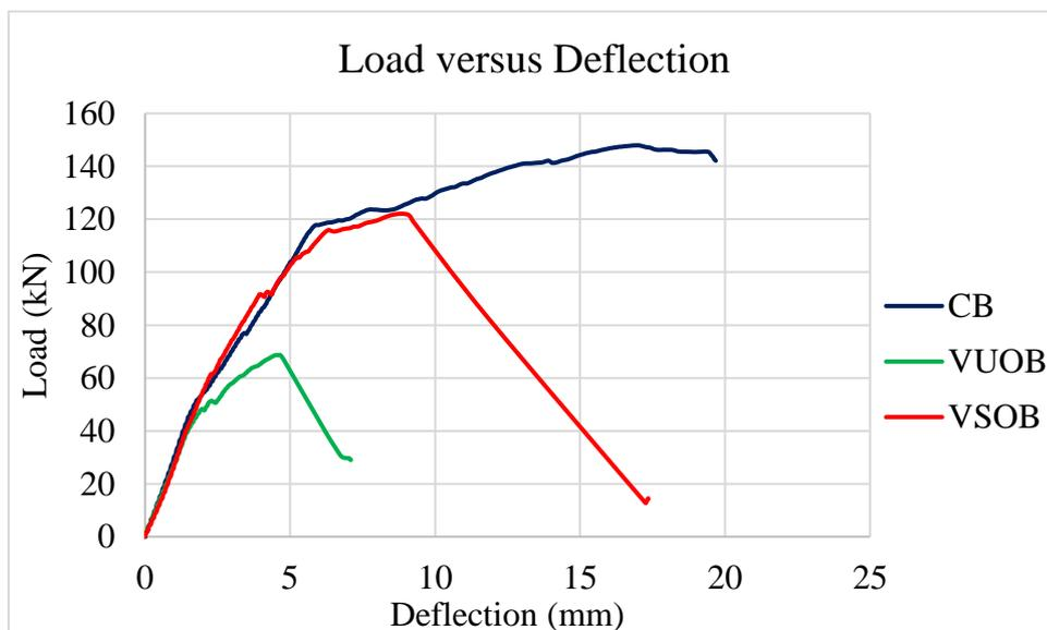
**Figure 4.22:** Load -deflection curve of circular opening beams.
