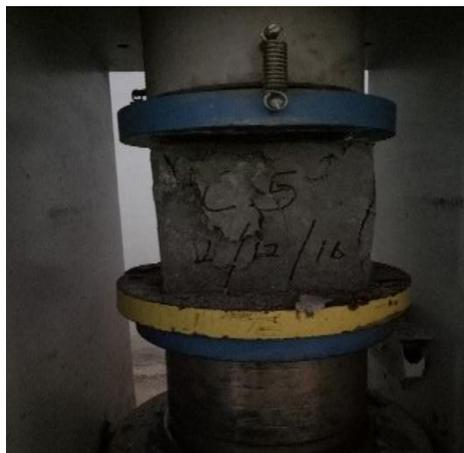
**Figure 4.2:** Compression test
