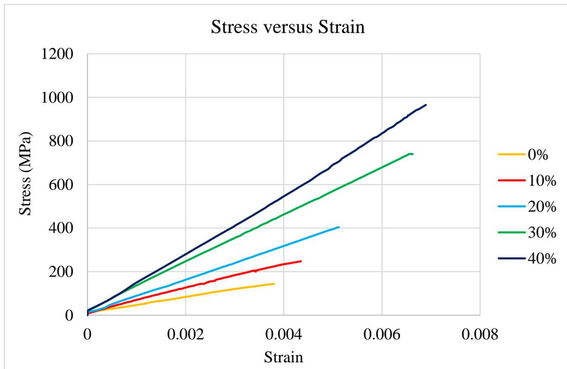
**Figure 4.16:** Comparison of stress versus strain in tensile test.
