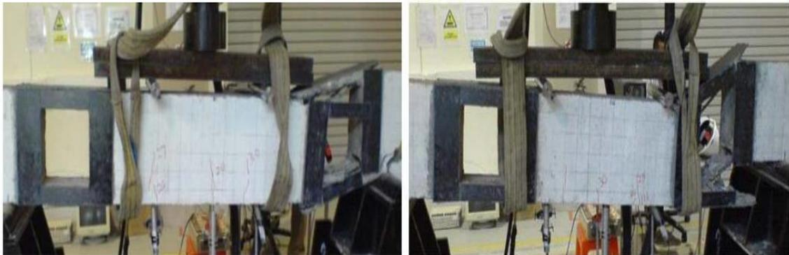
**Figure 2.19:** Cracks pattern and failure mode of strengthened beams with rectangular openings
