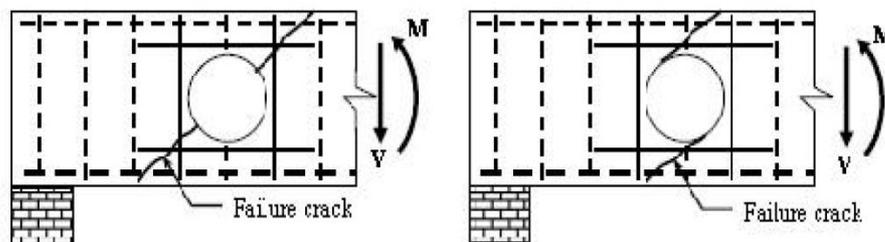
**Figure 2.15:** Beam-type failure and frame-type failure.
