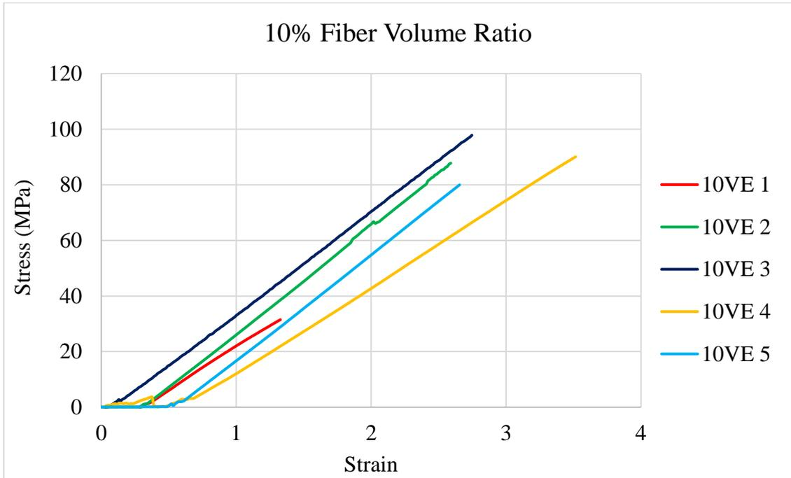
**Figure 4.6:** Stress versus Strain curve in flexural test 10% fiber volume ratio.
