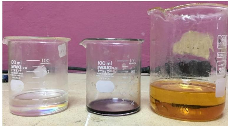
**Figure 3.5:** Matrix polymer. (Vinyl Ester, Cobalt Accelerator, Hardener MEKP)
