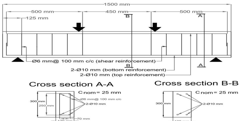
**Figure 3.13:** Arrangement of reinforcement bars in solid RC beam
