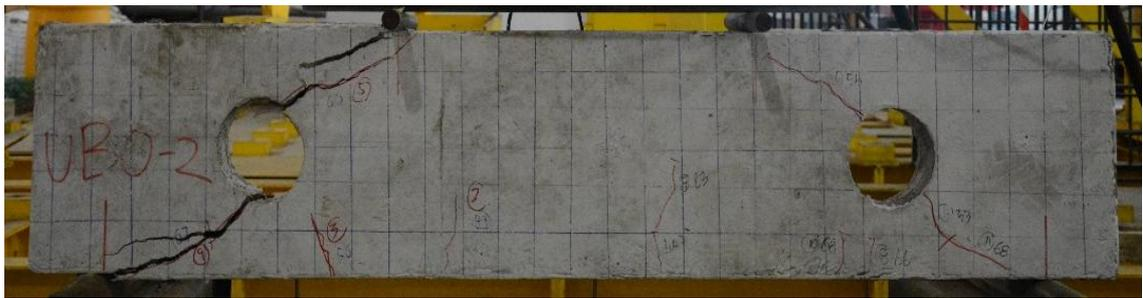
**Figure 4.24:** Crack pattern after failure for un-strengthened circular openings beam (VUOB)
