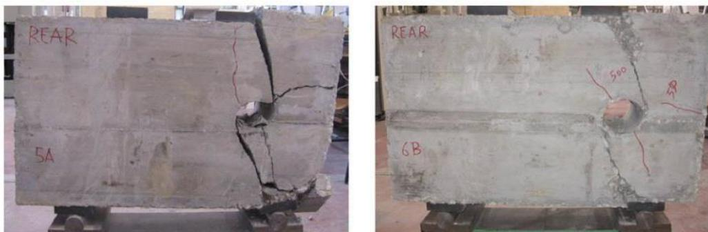
**Figure 2.14:** Specimens with openings in the shear-span after testing
