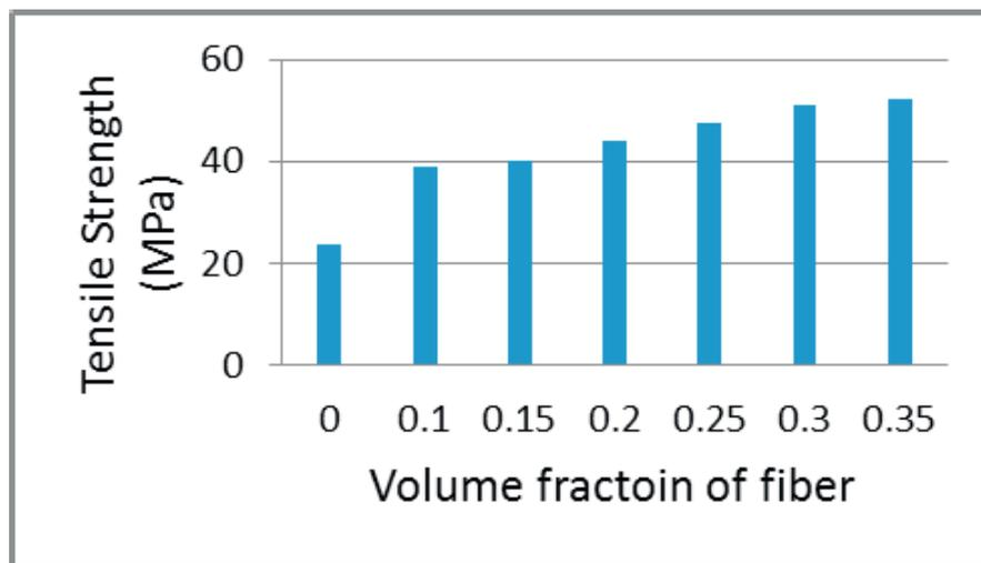
**Figure 2.7:** Effect of volume fraction of fiber towards tensile strength in composite plate.
