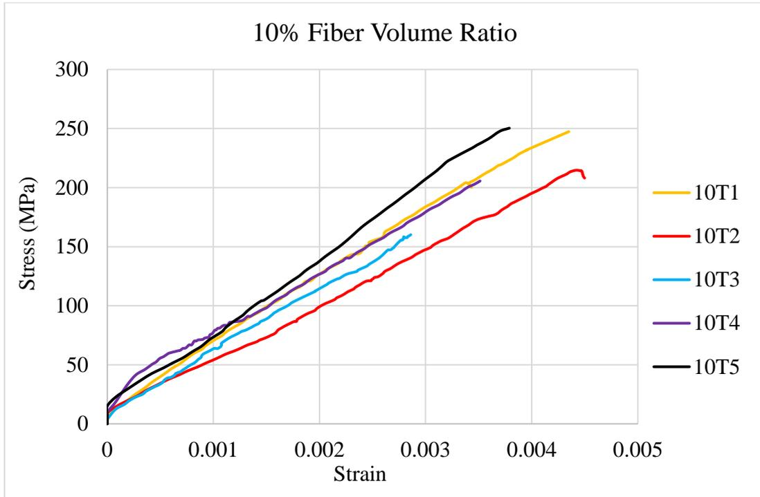
**Figure 4.12:** Stress versus Strain curve in tensile test with 10% fiber volume ratio.
