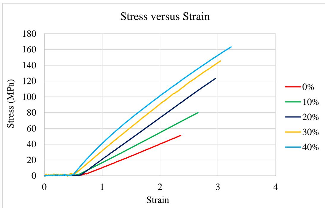
**Figure 4.10:** Comparison of stress versus strain in flexural test.
