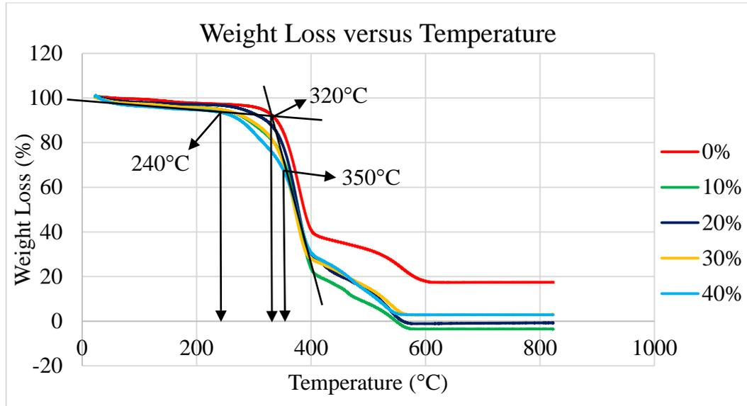
**Figure 4.17:** Weight versus Temperature graph of TGA.
