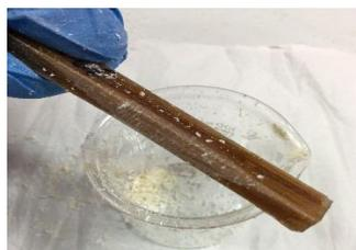
**Figure 3.27:** Shaved BFRCP for FTIR test
