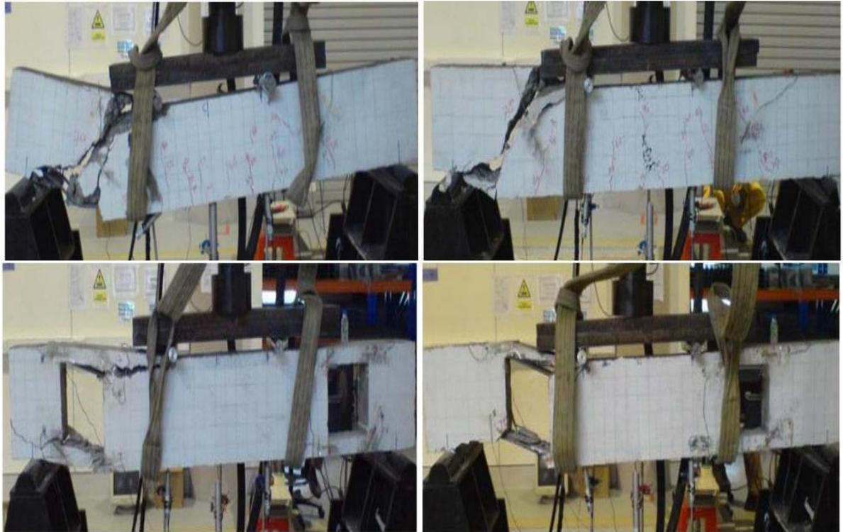
**Figure 2.17:** Cracks pattern and failure mode of control beam and un-strengthened beams with rectangular openings
