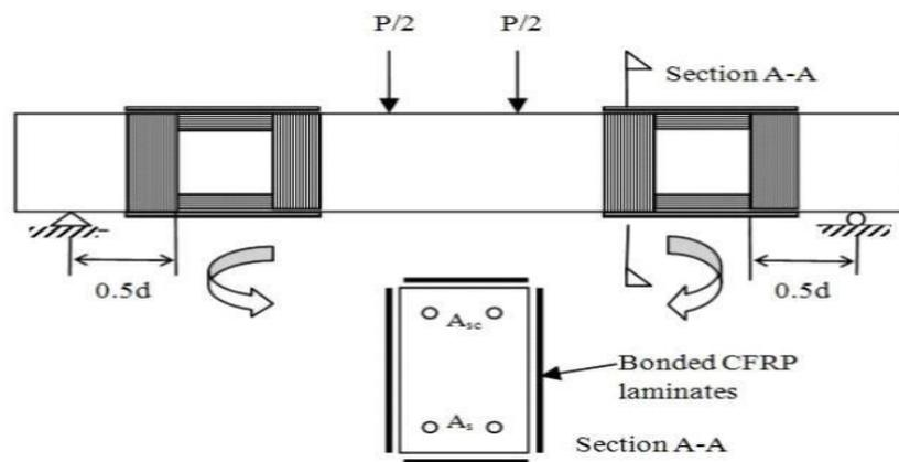
**Figure 2.18:** CFRP strengthening configuration by Chin et al.
