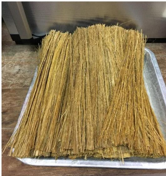
**Figure 3.2:** Processed individual bamboo fiber
