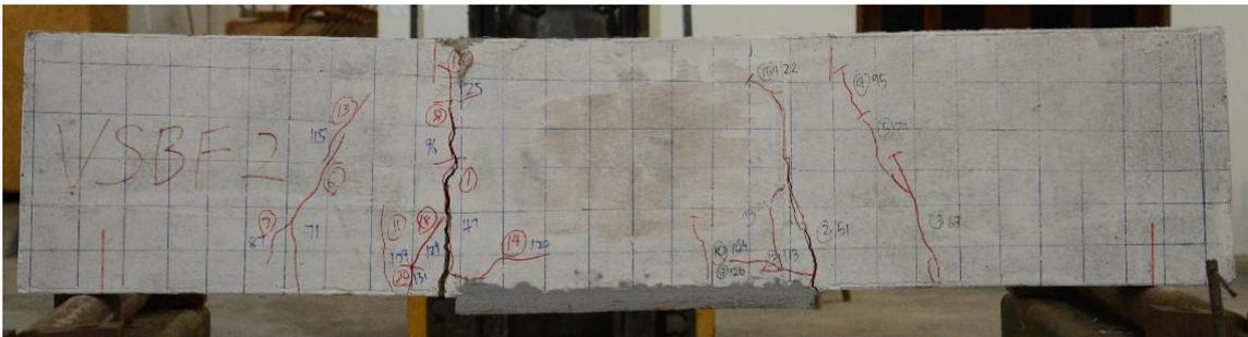
**Figure 4.21:** Crack pattern after failure for strengthened solid beam (VSSB)
