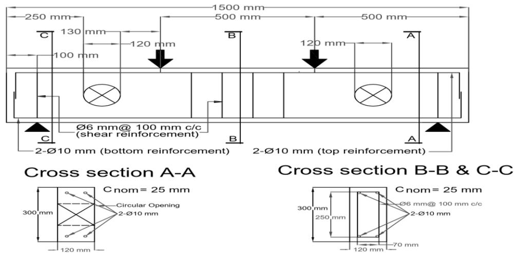
**Figure 3.14:** Arrangement of reinforcement bars in RC beam with circular opening
