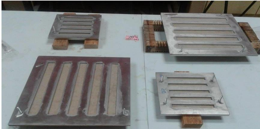
**Figure 3.8:** Stainless steel moulds for composite fabrication
