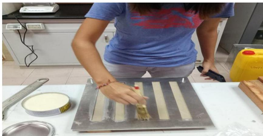
**Figure 3.9:** Application of mould releasing agent (honey wax)
