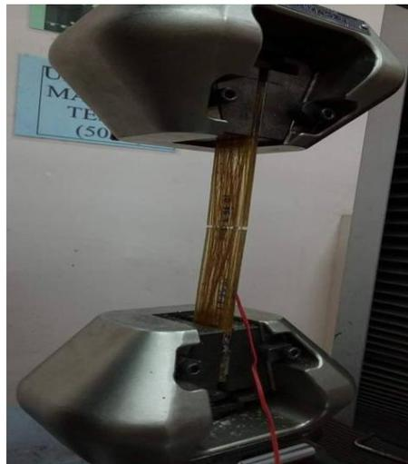
**Figure 3.29:** Tensile test for composite plate
