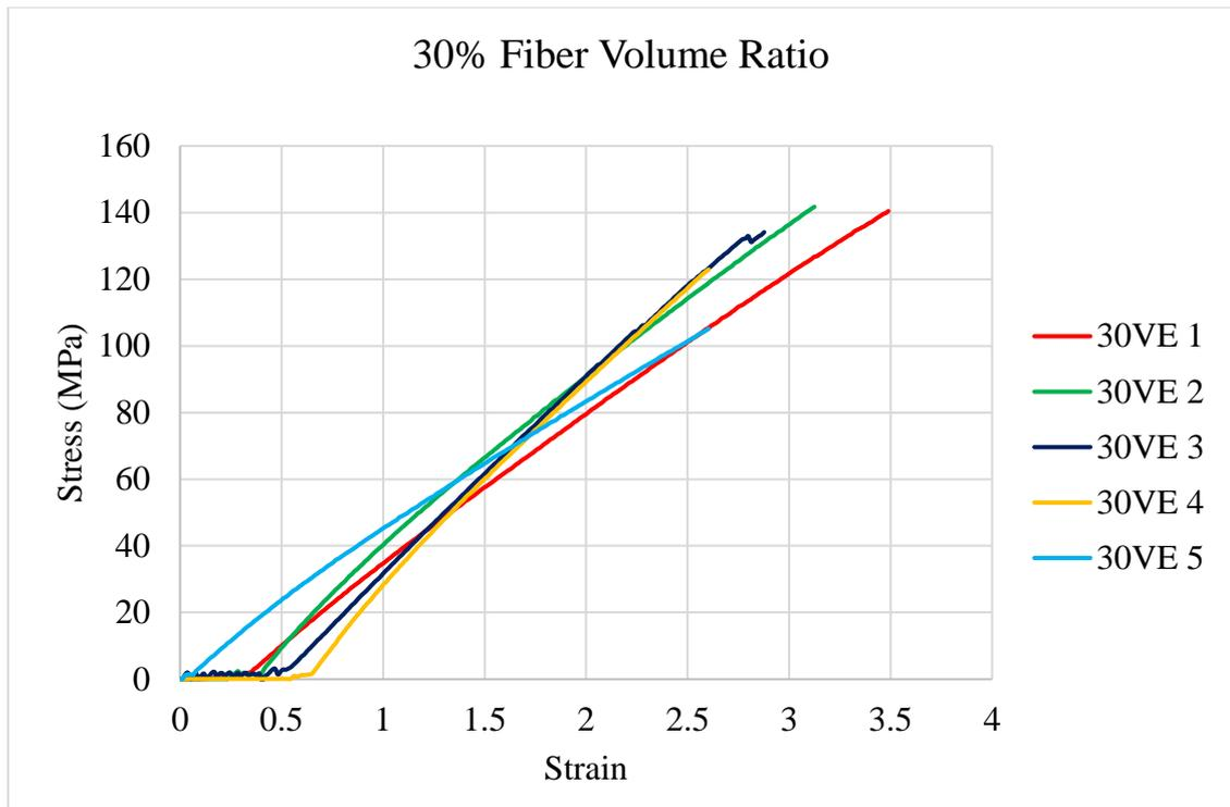
**Figure 4.8:** Stress versus Strain curve in flexural test with 30% fiber volume ratio.
