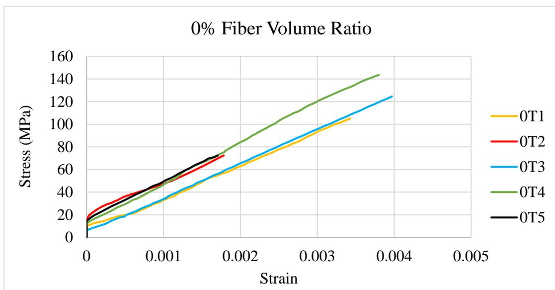
**Figure 4.11:** Stress versus Strain curve in tensile test with 0% fiber volume ratio.
