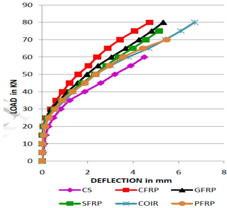
**Figure 2.12:** Comparison of different fiber sheet and control specimen in terms of deflection
