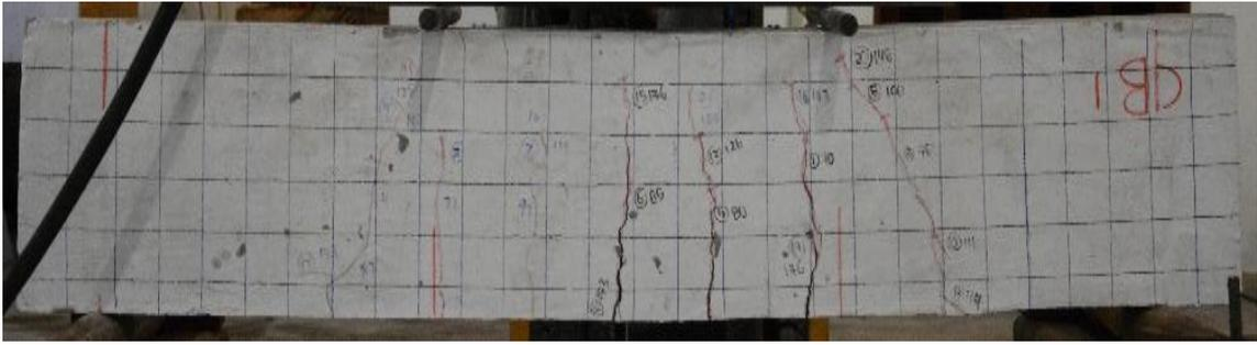
**Figure 4.19:** Crack pattern after failure for control beam (CB)
