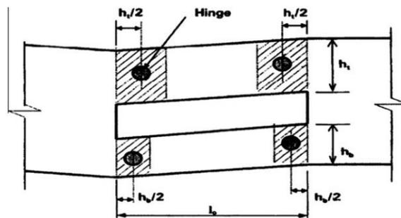
**Figure 2.16:** Forming of hinge in RC beam with opening.
