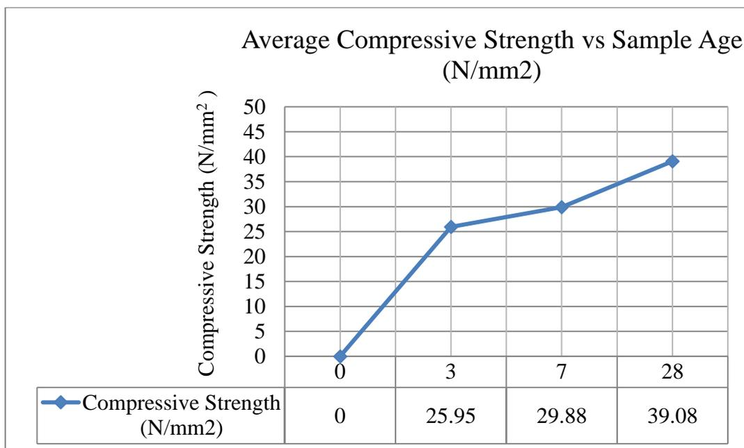
**Figure 4.3:** Graph of compressive strength versus days
