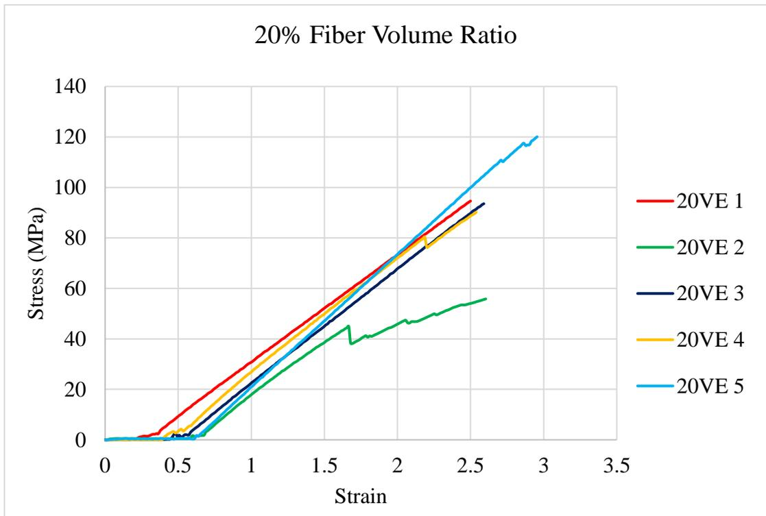
**Figure 4.7:** Stress versus Strain curve in flexural test with 20% fiber volume ratio.
