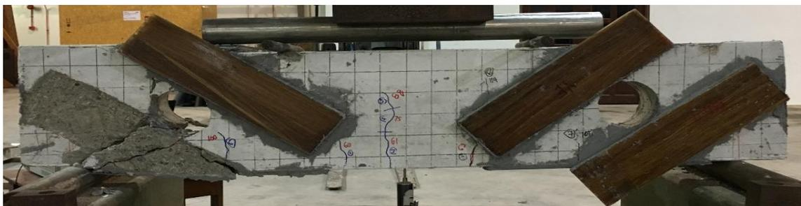
**Figure 4.25:** Crack pattern after failure for strengthened circular openings beam (VSOB)
