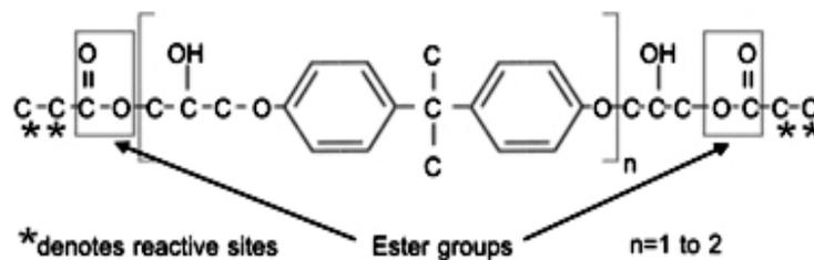
**Figure 2.4:** Chemical structure bonding of vinyl ester
