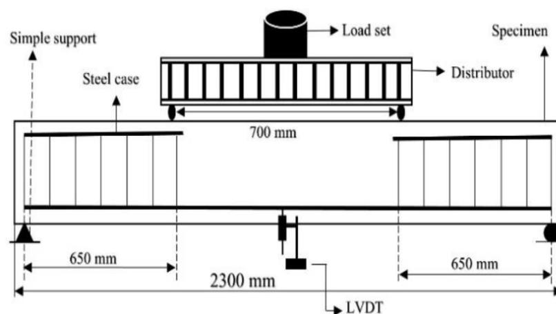
**Figure 2.10:** Three point loading Test.
