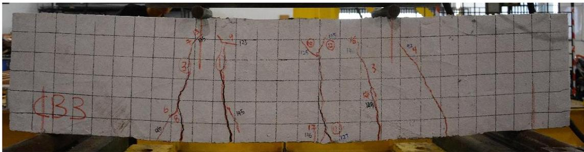
**Figure 4.23:** Crack pattern after failure for control beam (CB)
