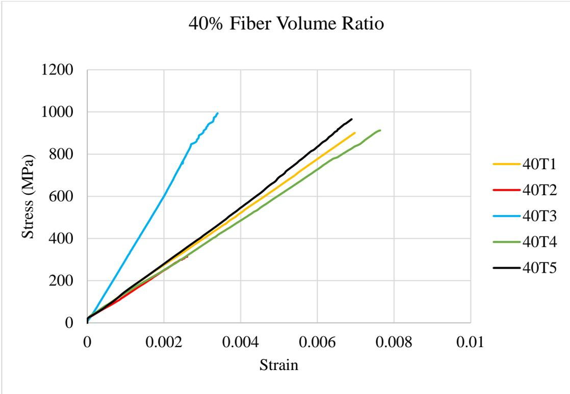
**Figure 4.15:** Stress versus Strain curve in tensile test with 40% fiber volume ratio.
