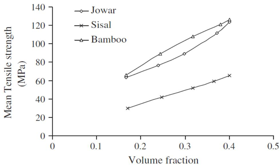
**Figure 2.9:** Effect of volume fraction of fibre for jowar fibre reinforced composites in comparison to sisal and bamboo fibre composites in tensile test.
