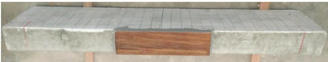
**Figure 3.23:** BFRCP bonded at the mid-span soffit of RC solid beam
