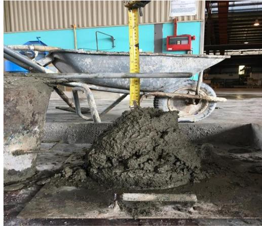
**Figure 3.31:** Slump test.
