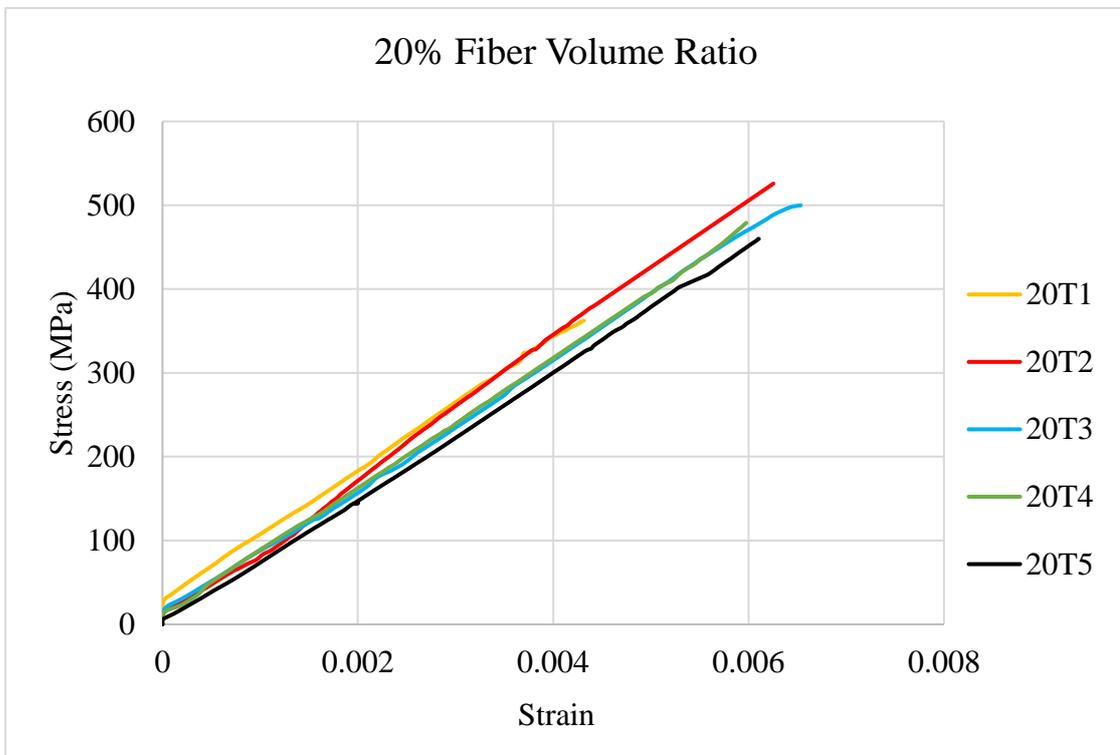
**Figure 4.13:** Stress versus Strain curve in tensile test with 20% fiber volume ratio.
