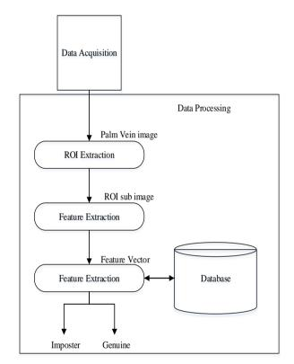
Figure 1: Process flow of the palm vein recognition system [1]
