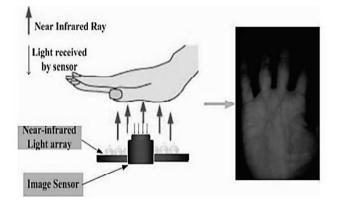
Figure 2: Basic principal of near infrared camera on capturing palm vein image [1]
