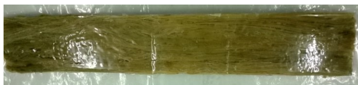
Figure 3. PALF-epoxy composite plate.
