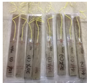
Figure 2. Composite samples with different fiber volume ratios.
