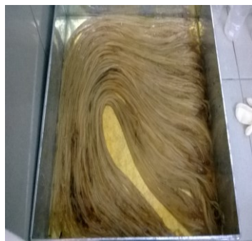
Figure 1. Fibers treated in NaOH solution.
