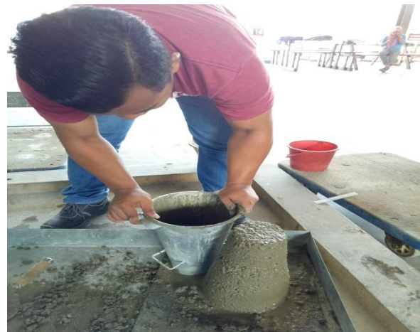
Figure 3 : Slump test in progress
