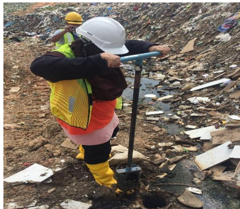
Figure 3.2.1 Sample collection using hand auger
