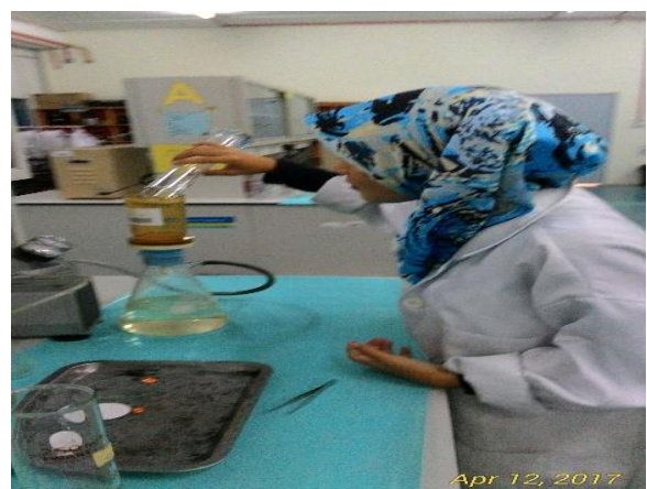
Figure C6: Total Suspended Solid test
