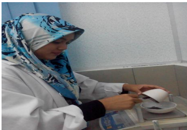
Figure C9: Weight the activated carbon
