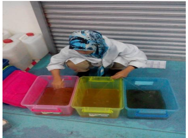
Figure C4: Stir sample with activated carbon
