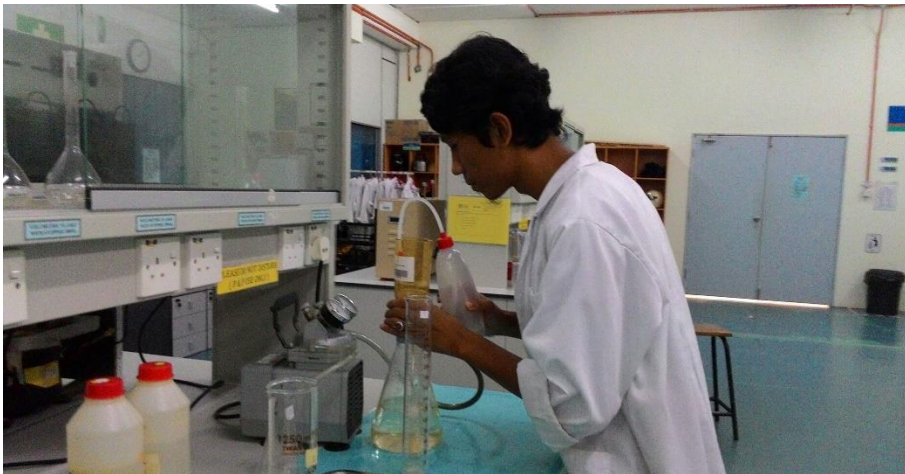
Figure F5: Total suspended solid test
