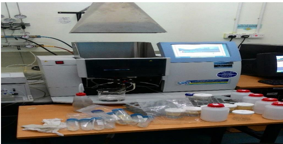
Figure F6: Atomic Absorption Spectrophotometric method
