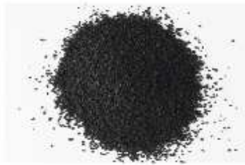
Figure 3.4 Crumb rubber powder 0.3mm-0.6mm (30 mesh)
