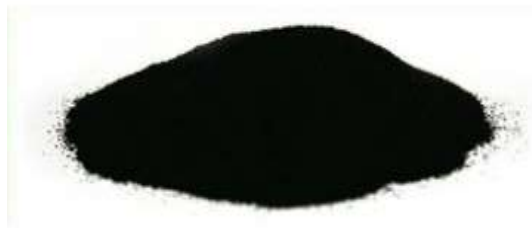
Figure 2.1 Crumb rubber powder (0.3mm – 0.6mm) Source: Wikipedia (2016)
