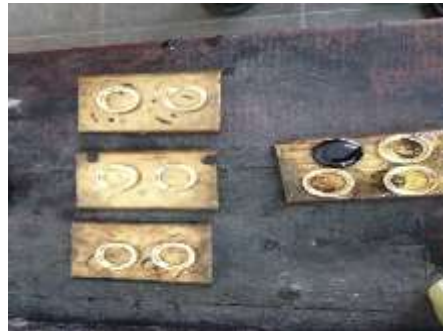
Figure 3.7 Four pairs of rings were placed into the plate which are unmodified bitumen, 1% of CR, 2% of CR and 3% of CR
