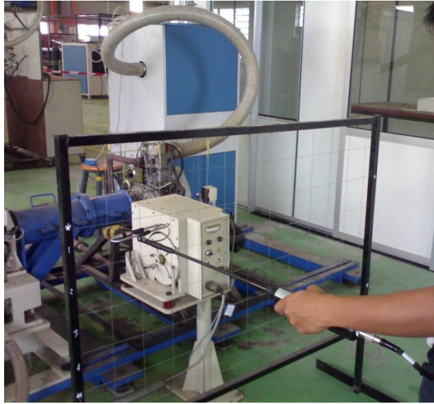
Figure 3.6: Noise sound identification setup using sound intensity method
