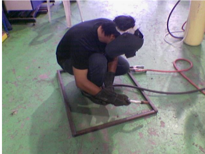
Figure 3.4: Welding process to make the Intensity Mesh
