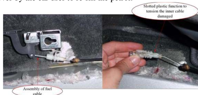
Figure 3. Example of damage assembly of fuel cable.
